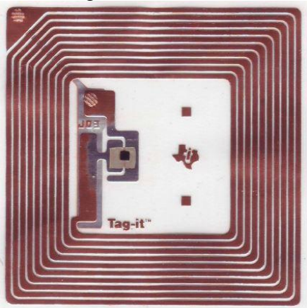
Figure 3.5 A passive RFID tag that is compatible with NFC [6]
