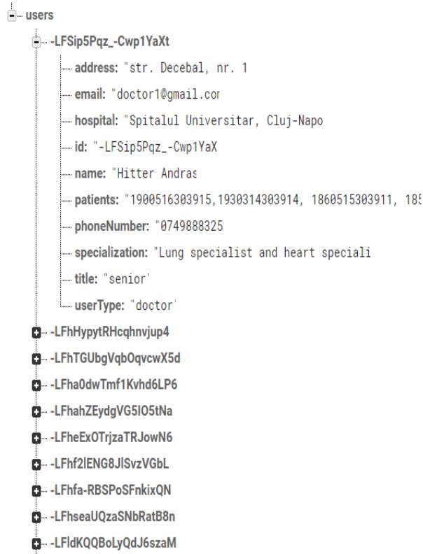
Figure 4.10 - Real-time Database structure
