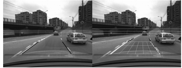
Fig. 4. Updating the clothoidal lane profile from linear segments using the Extended Kalman Filter
