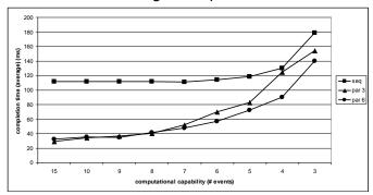
Figure 5-15: Completion time in relation to computational capability, homogeneous scenario
