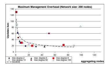
Figure 4-11: Management overhead incurred by A-GAP as a function of the number of aggregating nodes (degree of decentralization) for different aggregation tree degrees
