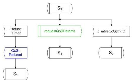
Figure A-6: QoSdmFC, state S3: bottom-up cross-layer request
