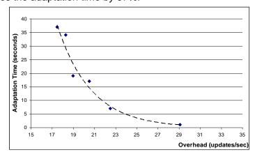
Figure 4-10: Adaptation time as a function of the incurred overhead for a network of 200 nodes
