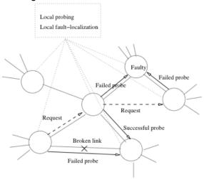
Figure 4-18: When a probe fails, the probing node asks neighbouring nodes for assistance in order to identify whether it is the probed node or the link that causes the anomaly.
