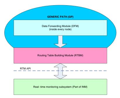
Figure 4-13: Generic Path and architecture of routing subsystem of 4WARD networks
