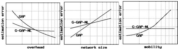
Figure 4-4: Comparison of tree-based (GAP) and gossip-based (G-GAP-NL) protocols for realtime monitoring: qualitative results from simulation study
