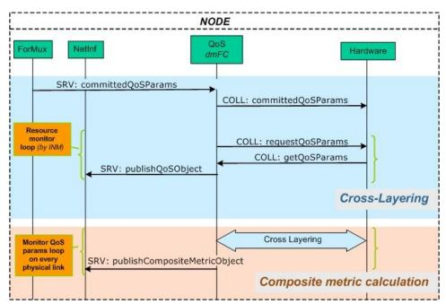
Figure 3-16: Example of exchanged messages between functional components (cf. Annex A)
