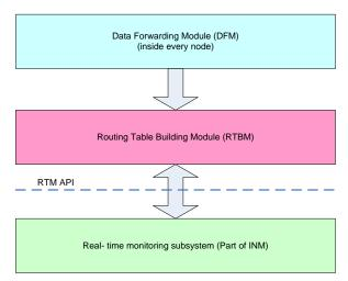
Figure 4-12 Generic decomposed architecture of routing subsystem in 4WARD networks
