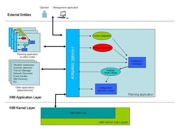
Figure 5-12: Architecture and external interfaces of the Network Configuration Planning application
