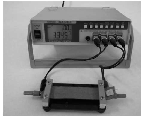
Figure 7. Fibre resistance measurement diagram.
