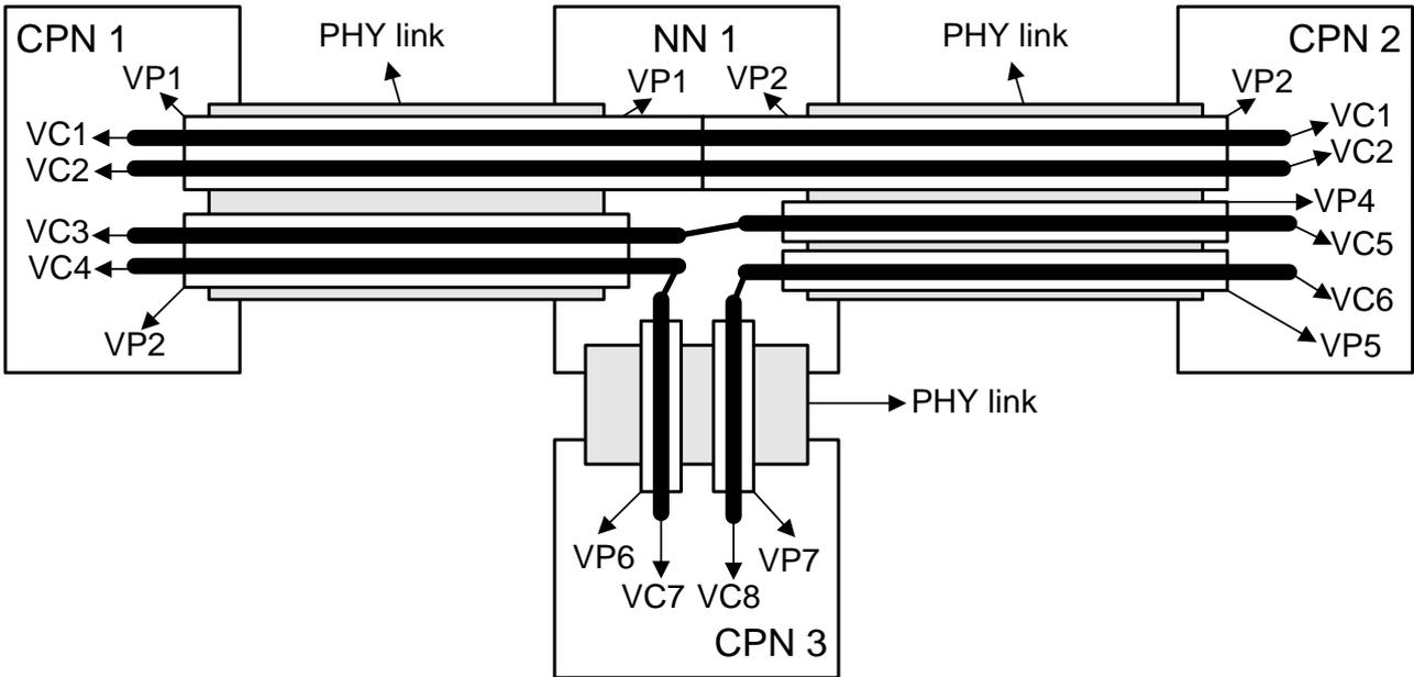
ATM Circuit and Path Connections
