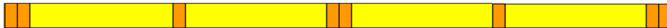
(b) Multiple short training blocks used for channel estimation and cyclic prefixes
