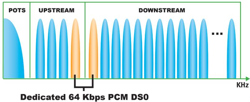
ates the need for packetization of voice traffic over the phone line into higher protocols such as ATM and IP (Figure 7). Multiple voice lines can be active simultaneously; given typical constraints on ADSL upstream bandwidth, four uncompressed voice lines might be a reasonable maximum, using an upstream bandwidth of 256 kbps.
