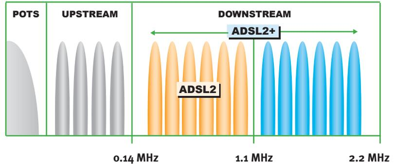
FIGURE 9: ADSL2+ DOUBLES THE MAXIMUM DATA RATE.
