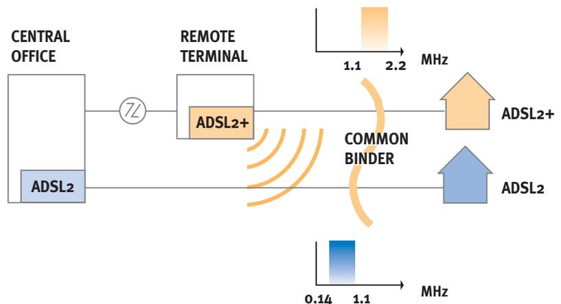
ADSL2+ can correct this problem by using frequencies below 1.1 MHz from the central office to the remote terminal, and frequencies between 1.1 MHz and 2.2 MHz from the remote terminal to the customer premise. This will eliminate most of the crosstalk between the services and preserve data rates on the line from the central office.
