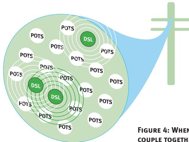
**FIGURE 4: WHEN ADJACENT PAIRS COUPLE TOGETHER THEY CAN CAUSE CROSSTALK, POTENTIALLY FORCING THE ADSL SYSTEM TO DROP A CONNECTION.**
