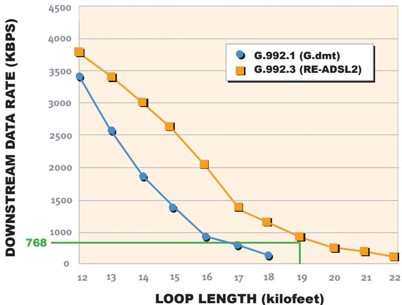
The Reach-Extended ADSL2 system was evaluated under a large number of crosstalk conditions and loop topologies [1,2,3]. Figure 12 compares the downstream data rate performance of conventional ADSL systems based on G.992.1 (G.dmt) and RE-ADSL2 systems based on G.992.3. The crosstalk environment for this
