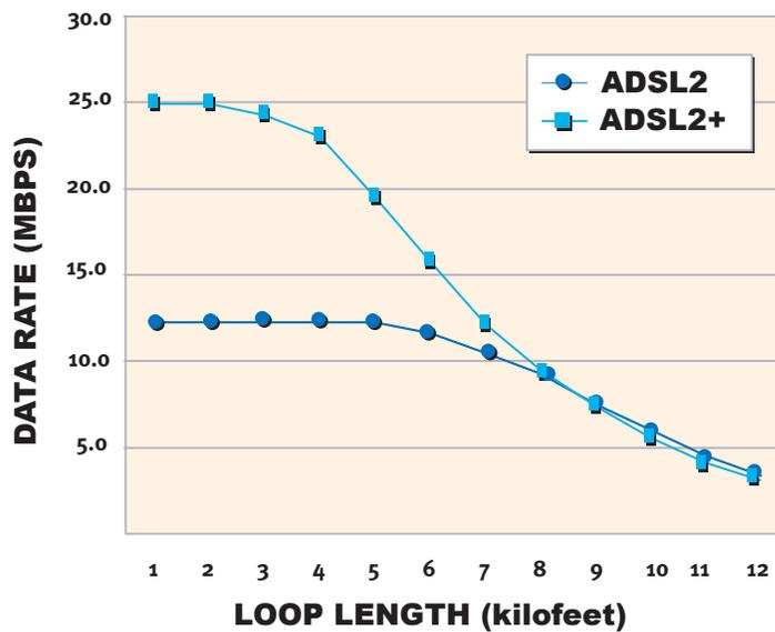
FIGURE 10: ADSL2+ CAN BE USED TO REDUCE CROSSTALK.
