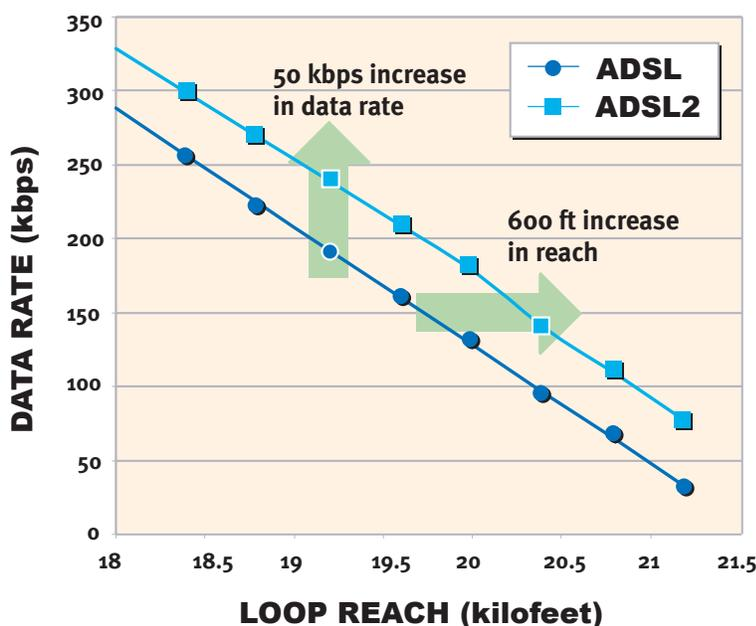
Figure 2 shows the rate and reach of ADSL2 as compared to the first-generation ADSL standard. On longer phone lines, ADSL2 will provide a data rate increase of 50 kbps; a significant increase for those customers who need it most.
