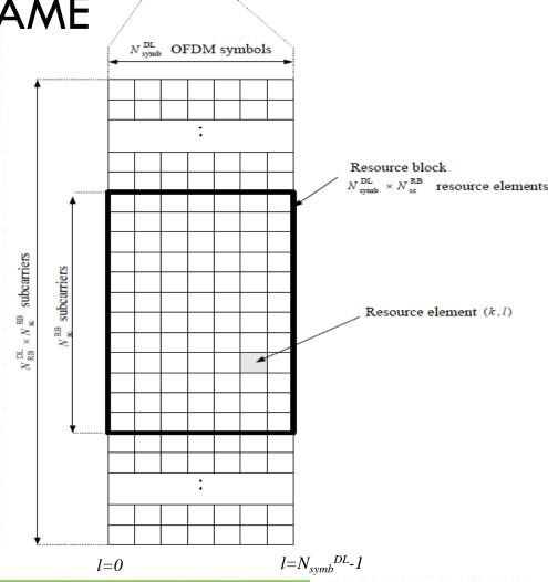
One downlink slot  $T_{slot}$
