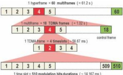
1 time slot = 510 modulation bits durations (~ 14.167 ms)
