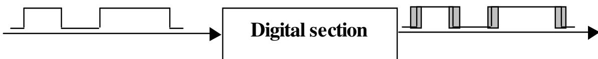
Fig. 21 Jitter phenomenon, which can be observed at the output of digital sections
