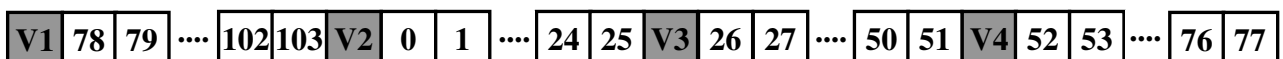
Fig. 15 Structure of the TU11 pointer and his position in this unit. Numbering of the TU11 unit positions
