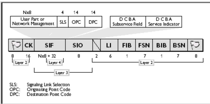
Fig. 14 SIF and SIO field structures
