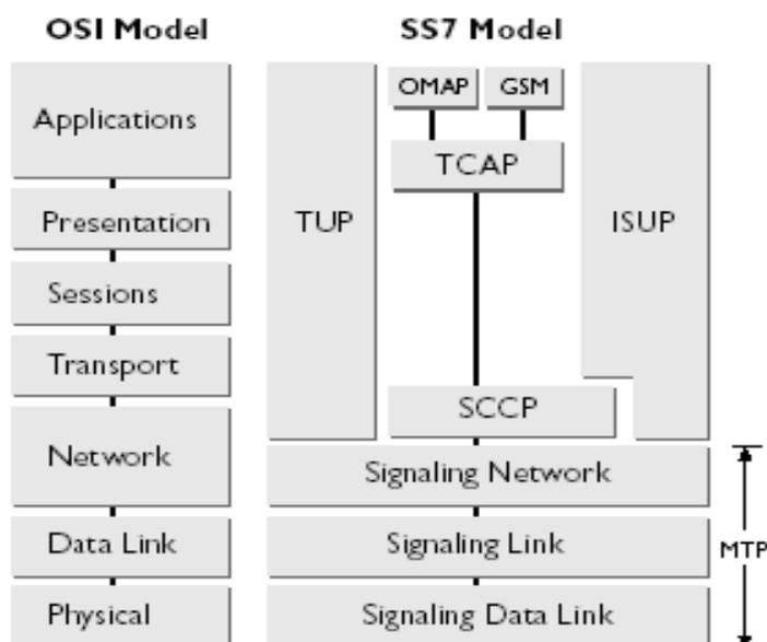
Fig. 7 The layers of SS7 protocols and comparison with the OSI layers
