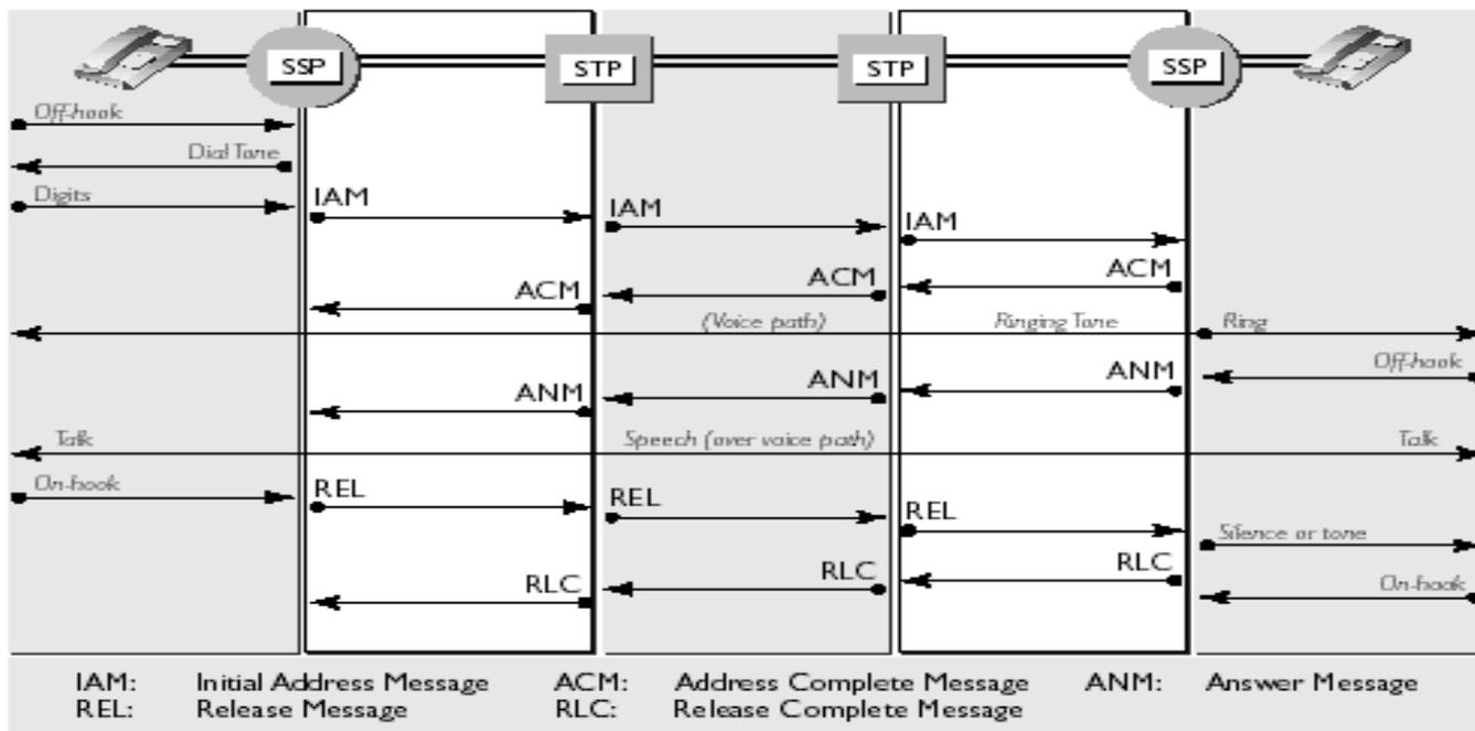
Fig. 5 Basic call setup based on SS7 signaling – alternative representation
