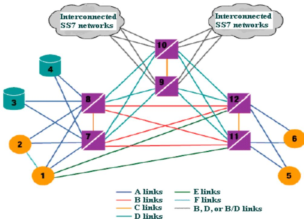
Fig. 3 Signaling link types used in SS7 networks
