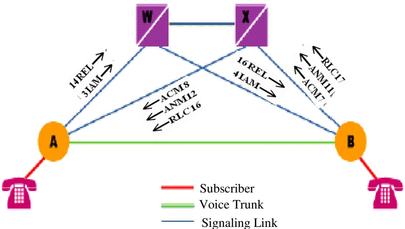
Fig. 4 Basic call setup based on SS7 signaling
