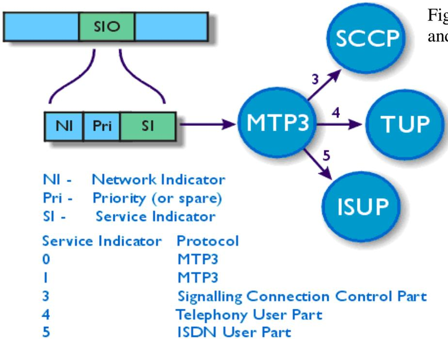
Fig. 13 Structure of the SIO octet and MTP3 message distribution
