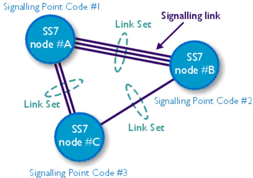
Fig. 11 Example of SS7 network and signaling link sets
