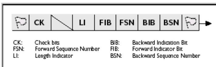
Fig. 8 FISU message structure
