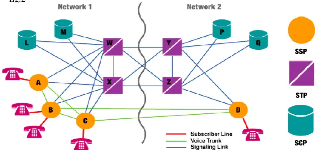
Fig. 2 The general structure a digital telephone network using SS7 signaling
