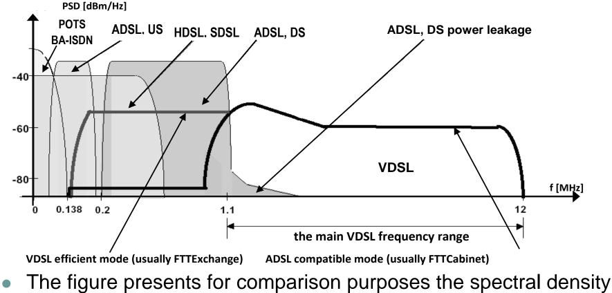
of the telephone and of the BA-ISDN signals;
