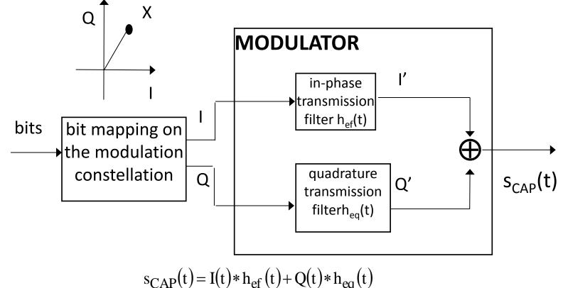
Conditions imposed to the transmission and reception filters transfer functions: |H<sub>ef</sub> (ω) = |H<sub>eq</sub> (ω) ∀ω
