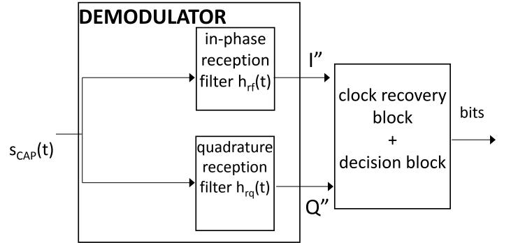
$I''(t) = s_{CAP}(t) * h_{rf}(t) = (I(t) * h_{ef}(t) + Q(t) * h_{eq}(t)) * h_{rf}(t) = I(t) * (h_{ef}(t) * h_{rf}(t)) + Q(t) * (h_{eq}(t) * h_{rf}(t)) = I(t) * (h_{ef}(t) * h_{rf}(t)) = I(t) * (h_{ef}(t) * h_{rf}(t))$
