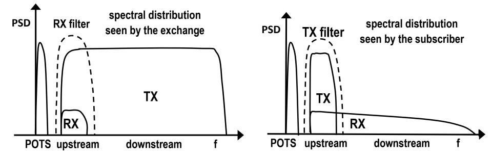
the figure indicates also the filtering characteristics and the transmission and reception signal levels.
