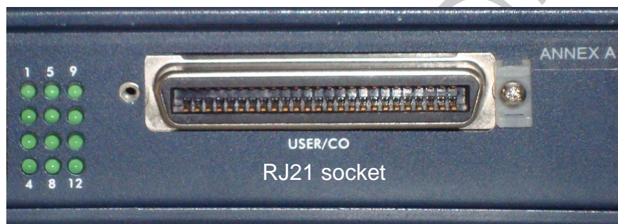
Figure 4.12: Connection panel of an ADSL2+ access multiplexer with 12 users made of an RJ21 connector.
