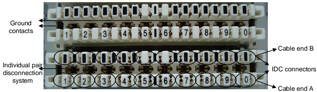
Figure 4.14: Krone type terminal strip with 10 pairs.
