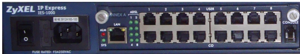
Figure 8.45: AAM-1008 DSLAM module installed in an IES-1000 rack.
