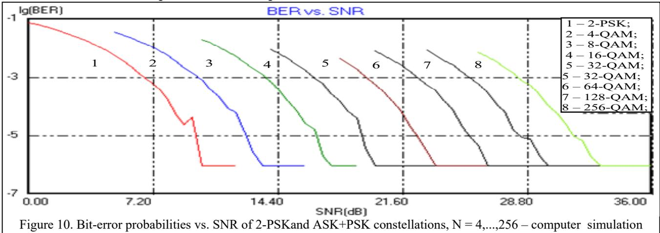
Figure 10. Bit-error probabilities vs. SNR of 2-PSK and QAM constellations, N = 4, ..., 256 – computer simulation
