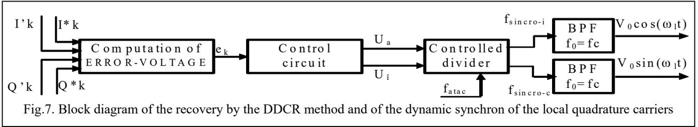
Fig.7. Block diagram of the recovery by the DDCR method and of the dynamic synchronon of the local quadrature carriers
