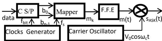
is applied to remove any undesired spectral components outside the allowed frequency band. Figure 1 presents the block diagram of an ASK transmitter; the figure doesn't contain the output BPF.
