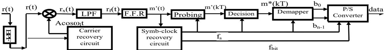
Figure 2 Block diagram of the ASK receiver
