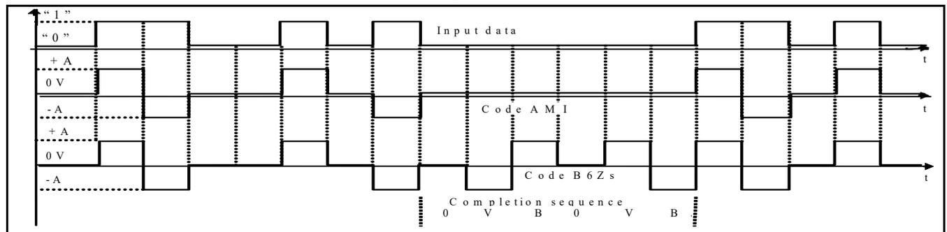
Figure 9. Encoding rules for the AMI and B6ZS codes
