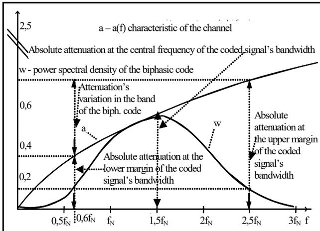
Figure 7. Effects of non-uniformity of the  $a(f)$  characteristic upon the biphasic-encoded signal
