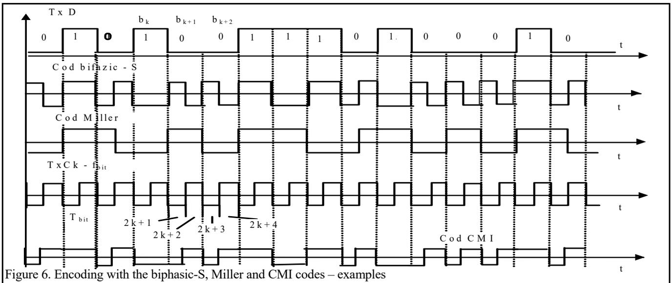
Figure 6. Encoding with the biphasic-S, Miller and CMI codes – examples
