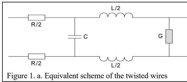
$$\gamma = \alpha(\omega) + j\beta(\omega); a = \alpha \cdot l; b = \beta \cdot l; Z_c(\omega) = \sqrt{\frac{R + j\omega L}{G + j\omega C}}; \quad (1)$$
