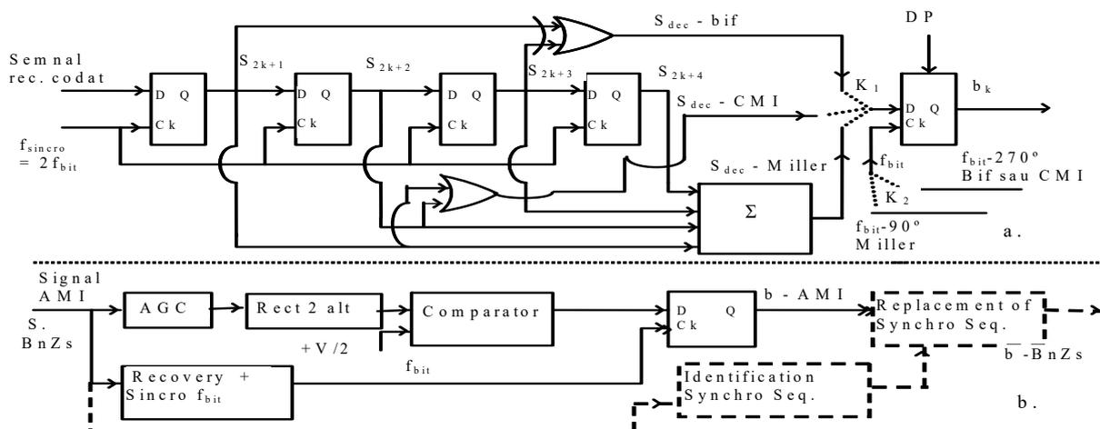
Fig. A2 a. Block diagram of the biphasic-S, CMI and Miller decoders; b. Block diagram of the AMI and BnZs decoders
