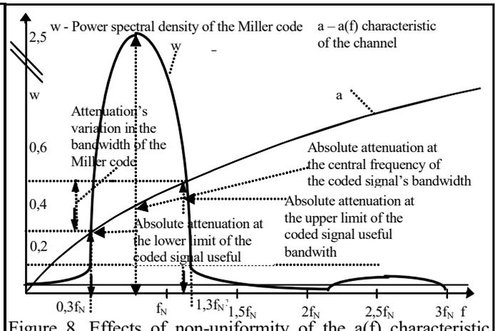
Figure 8. Effects of non-uniformity of the  $a(f)$  characteristic upon the Miller-encoded signal
