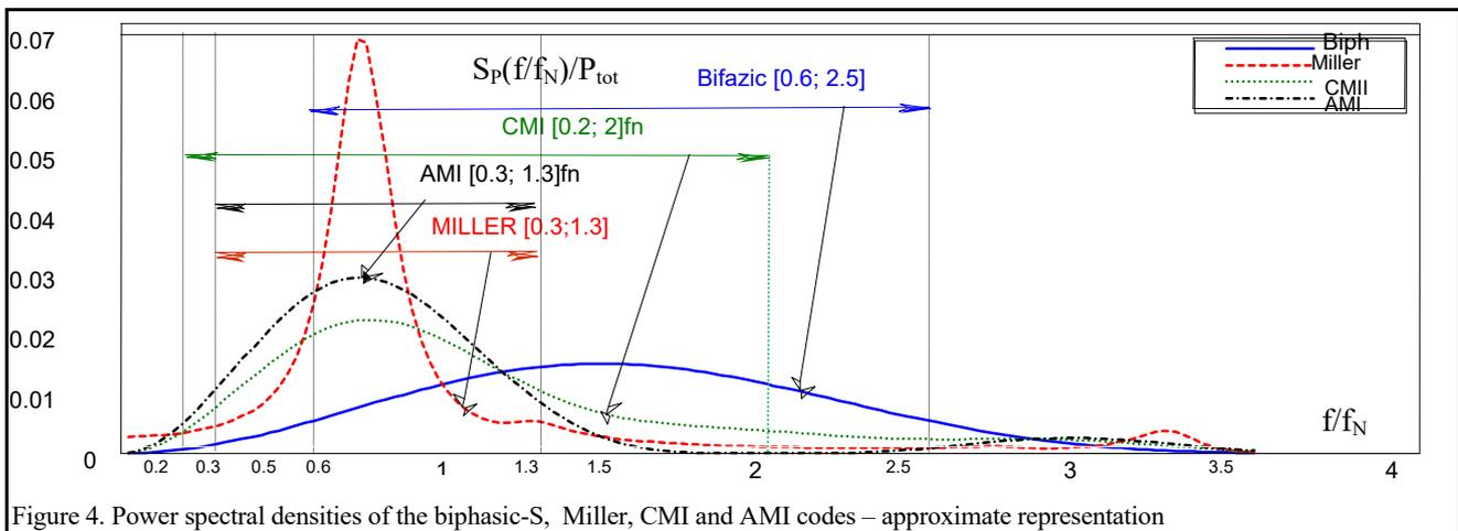
Figure 4. Power spectral densities of the biphasic-S, Miller, CMI and AMI codes – approximate representation
