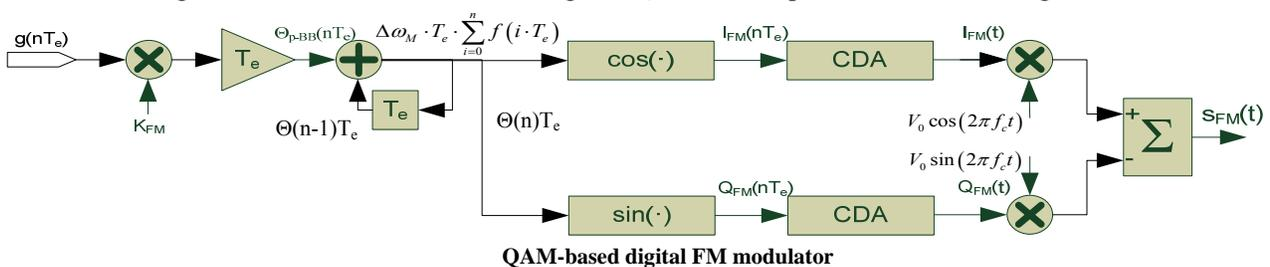
**Note:** the QAM based FM modulator requires a much smaller sampling frequency than the modulator that uses the digital generation of the FM signal directly on the carrier frequency (usually  $f_{mM} \ll f_c$ )
