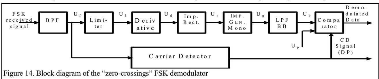
Figure 14. Block diagram of the “zero-crossings” FSK demodulator
