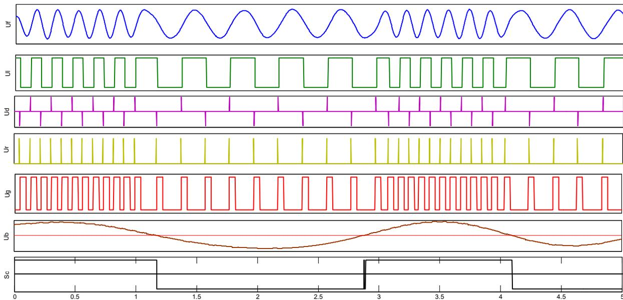
Figure 15. Signal diagram of the “zero-crossings” FSK demodulator
