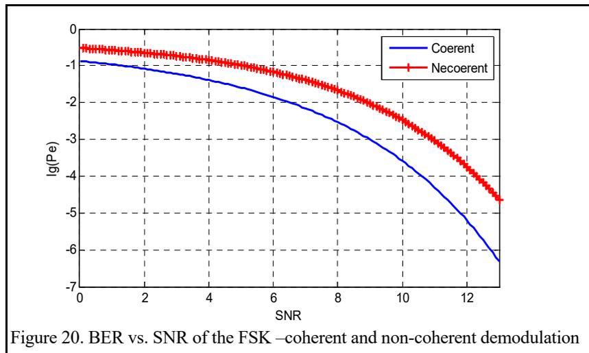
Figure 20. BER vs. SNR of the FSK –coherent and non-coherent demodulation
