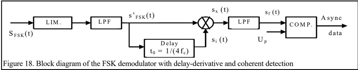
Figure 18. Block diagram of the FSK demodulator with delay-derivative and coherent detection
