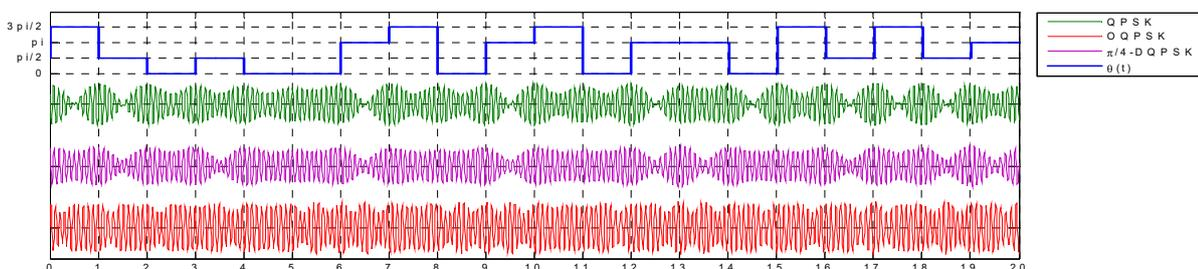
Figure 18. Envelope variations vs. time of QPSK, OQPSK and  $\pi/4$ -QPSK
