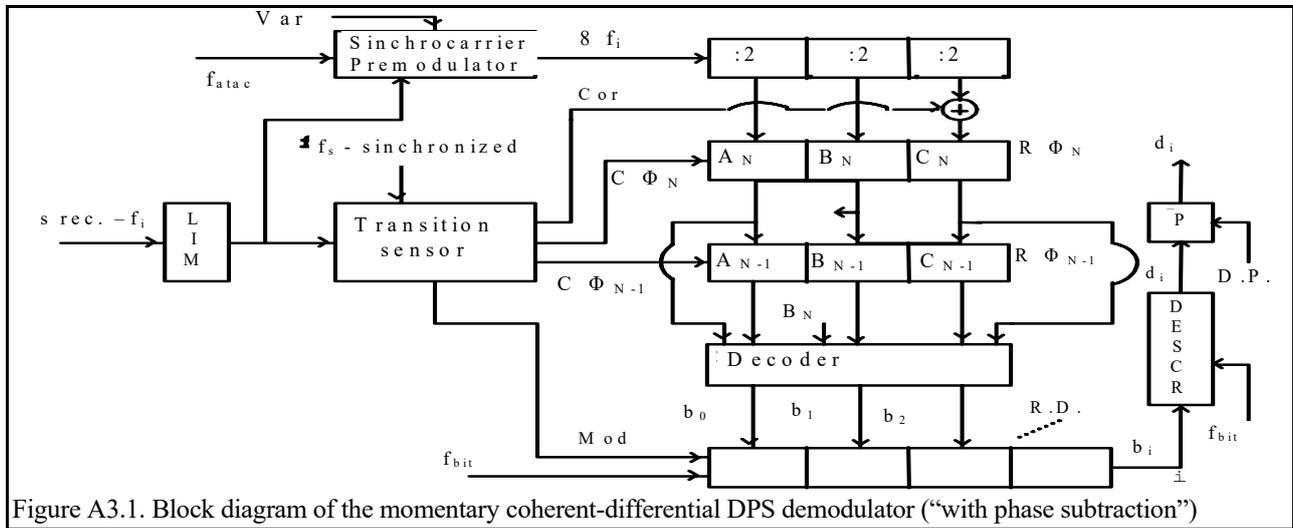
Figure A3.1. Block diagram of the momentary coherent-differential DPS demodulator (“with phase subtraction”)
