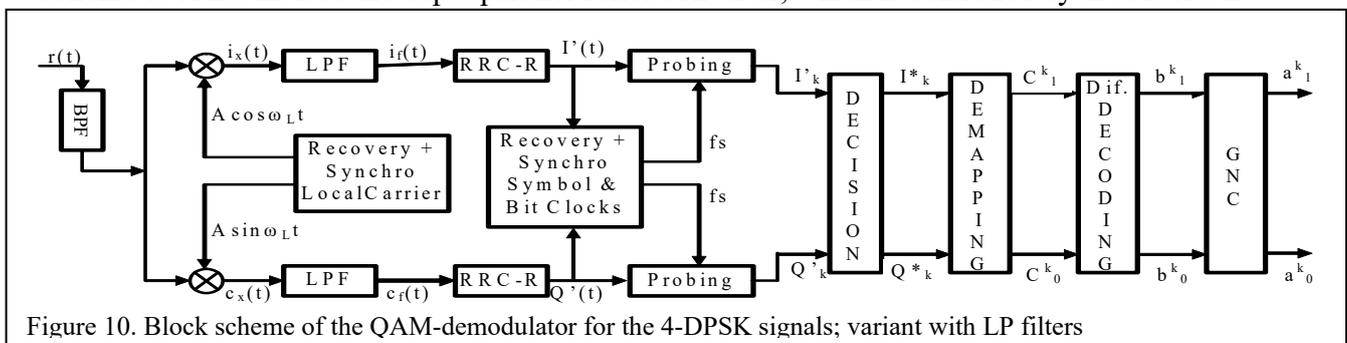
Figure 10. Block scheme of the QAM-demodulator for the 4-DPSK signals; variant with LP filters
