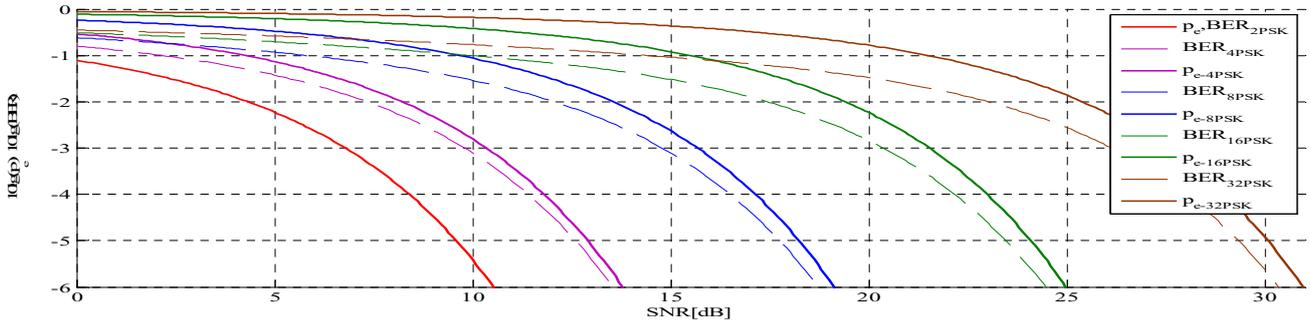
Figure 20.  $p_{e2}$ ,  $p_{e4}$ ,  $p_{e8}$ ,  $p_{e16}$ ,  $p_{e32}$  (continuous lines) and  $\text{BER}_2$ ,  $\text{BER}_4$ ,  $\text{BER}_8$ ,  $\text{BER}_{16}$ ,  $\text{BER}_{32}$ , (dashed lines) vs. SNR
