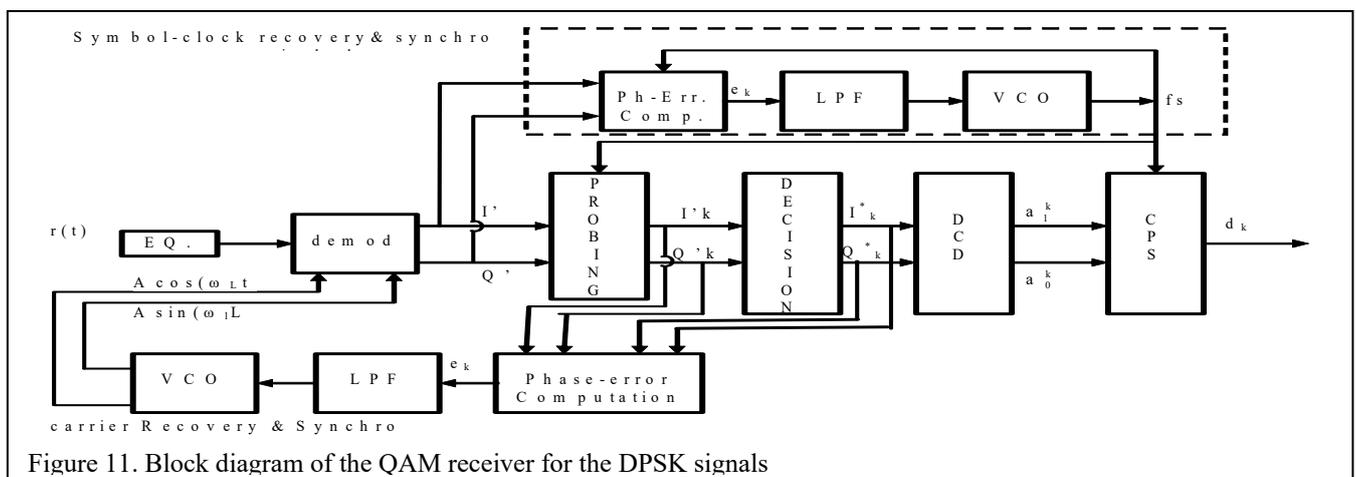
Figure 11. Block diagram of the QAM receiver for the DPSK signals
