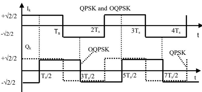
Fig. 14. Relative positioning of the  $I_k$  and  $Q_k$  modulating levels, to generate the QPSK and OQPSK modulations
