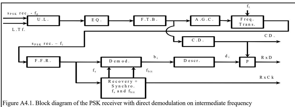
Figure A4.1. Block diagram of the PSK receiver with direct demodulation on intermediate frequency
