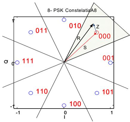
Fig. 19. Vectorial composition of the received signal
