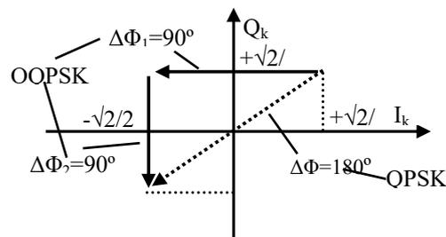
Fig. 15 Generation of the  $180^\circ$  phase-shifts by QPSK and OQPSK
