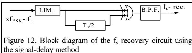
Figure 12. Block diagram of the  $f_s$  recovery circuit using the signal-delay method
