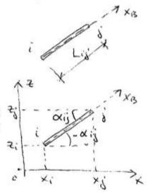
COMPARED TO THE & ARIS OF THE GOUDRAL REFERENCE SYSTEM, AND THE ENDPOINTS OF THE BEAM WILL RESULT WITH PAIRS OF COURDINATES PROJECTED ON BOTH ARES OF THE GENERAL REFERENCE SYSTEM (REPRESENTING ALSO THE COORDINATES OF THE PINNETS JOINTS OR NODES, CONNECTED THROUGH THE BEAM). THE ORIENTATION OF THE BEAM CAN BE EXPRESSED BY :
