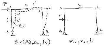
Considering the above frame loaded by the *P* force, the cross-section *i* will have a displacement (the horizontal component being marked as  $\Delta_i$ ). Thus, a virtual horizontal unit load can be considered (according to the direction of  $\Delta_i$ ) going through a real  $\Delta_i$  displacement. Starting from the expression of elastic static equilibrium (meaning null virtual mechanical work) of the structure:
