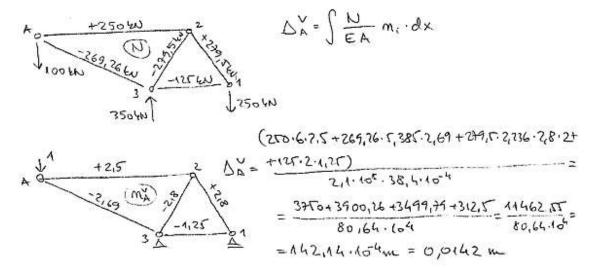
Since the axial force diagrams are rectangular, only the values of the forces were marked on the structural schemes.
