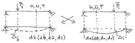
In other words, it can be considered a real  $P_j$  load producing a virtual displacements (also real forces with virtual displacements), or a virtual  $P_i$  load corresponding to a real displacement (also virtual forces with real displacements). This will lead to the conclusion, that multiplying the force with the displacement marked on the two figures below will result in the same mechanical work.
