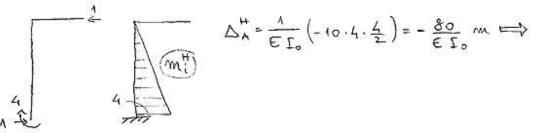
Since the resulted value is negative, the horizontal displacement will be towards right (opposed to the direction of the applied horizontal unit load).
