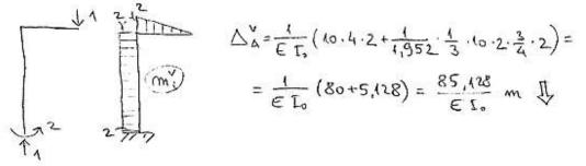
As it can be observed, the vertical displacement will be downwards (in the same direction as the applied vertical unit load).
