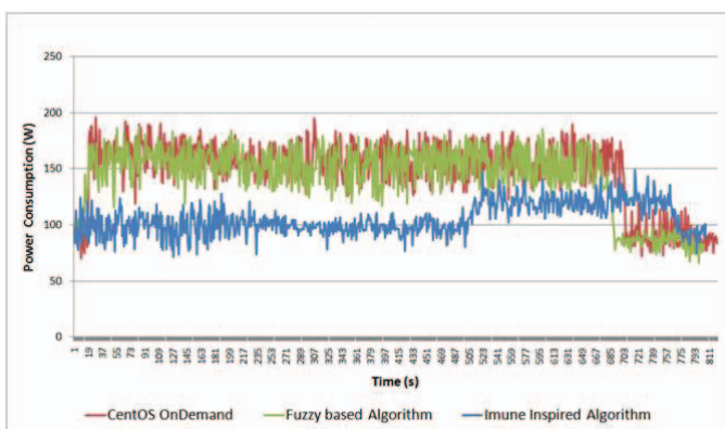
Figure 4. The server power consumption chart when executing the same CPU intensive workload with different management algorithms
