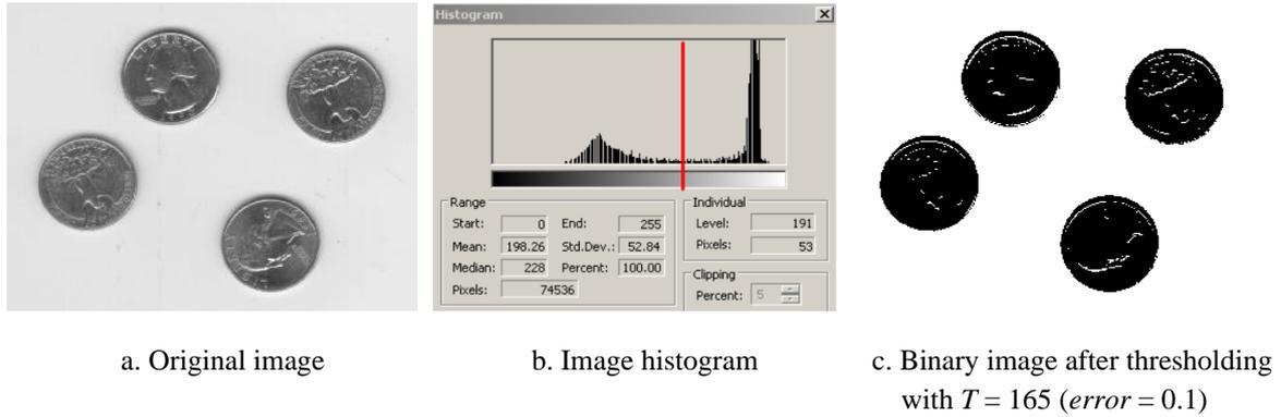
Fig. 8.14 Segmentation result using the computed threshold
