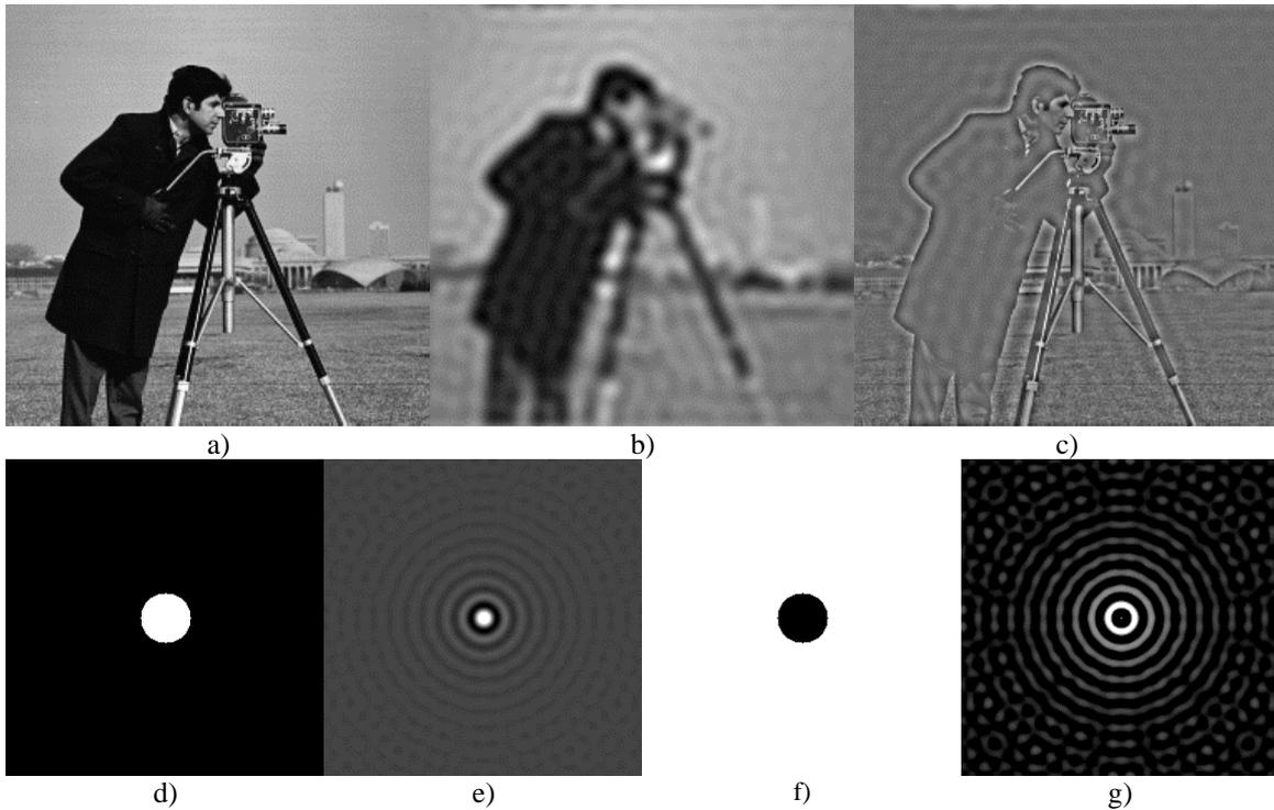
**Fig. 9.6** a) Original image; b) Result of ideal low-pass filtering; c) Result of ideal high-pass filtering; d) Ideal low-pass filter in the frequency domain; e) Corresponding ideal low-pass filter in spatial domain; f) Ideal high-pass filter in frequency domain; g) Corresponding ideal high-pass filter in the spatial domain ( $R=20$ )
