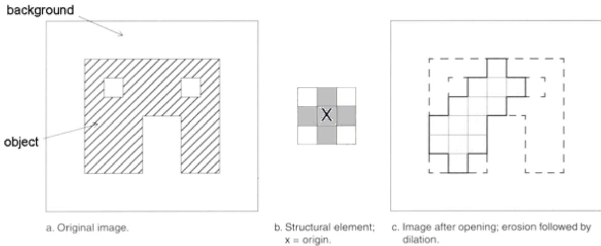
**Fig. 7.6** Illustration of the opening process [1]
