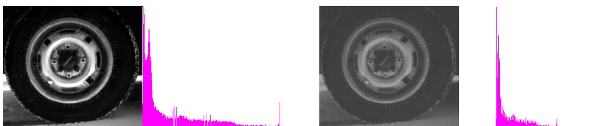
a. Original image and histogram      b. Histogram shrinking ( $g_{out}^{MIN}=50, g_{out}^{MAX}=150$ )
