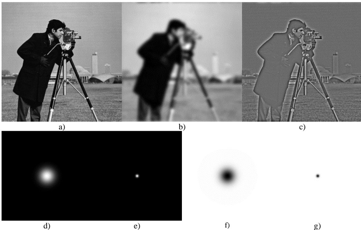
**Fig. 9.7** a) Original image; b) Result of Gaussian low-pass filtering; c) Result of Gaussian high-pass filtering; d) Gaussian low-pass filter in the frequency domain; e) Corresponding Gaussian low-pass filter in the spatial domain; f) Gaussian high-pass filter in the frequency domain; g) Corresponding Gaussian high-pass filter in the spatial domain ( $A=20$ )
