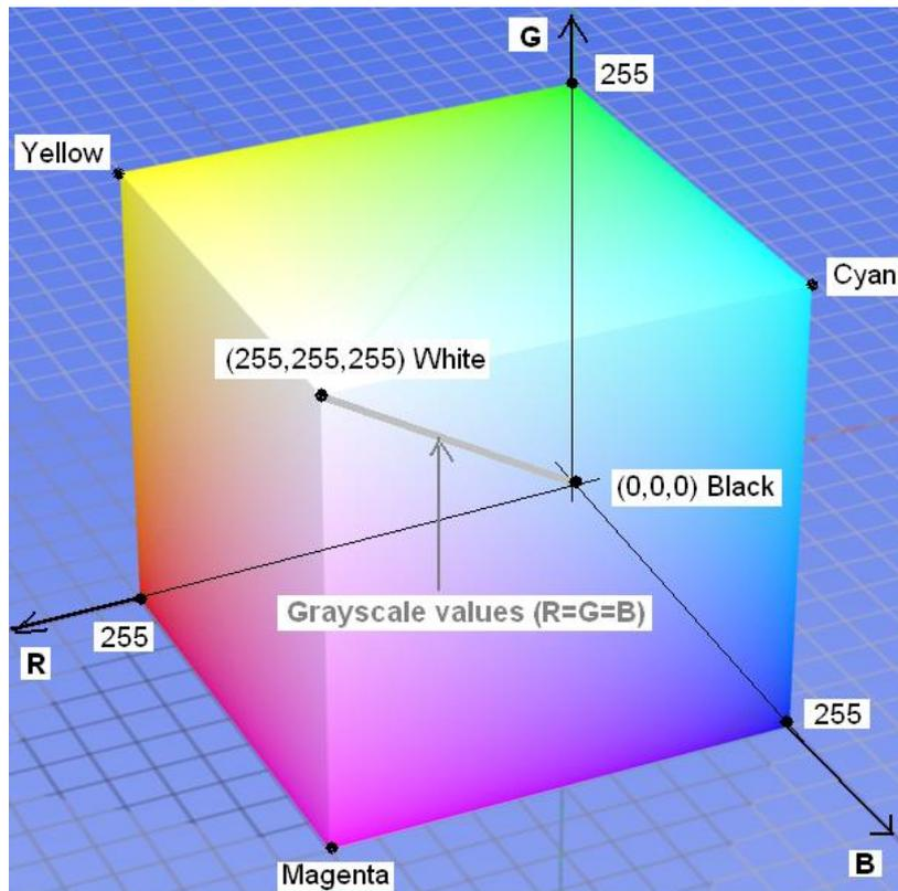
**Fig. 2.3** The RGB color space mapped on a cube. Here, each color axis is represented on 8 bits (256 levels) (RGB24 bitmap images). The total number of colors is  $2^8 \times 2^8 \times 2^8 = 2^{24} = 16.777.216$
