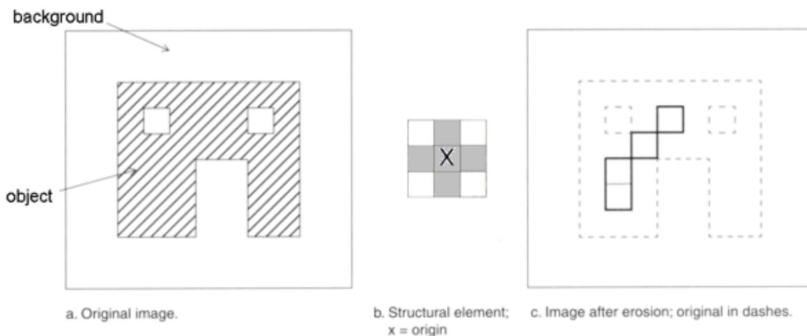
Fig. 7.4 Illustration of the erosion process [1]
