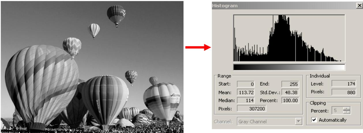
Fig. 3.1 Example: the histogram of a grayscale image
