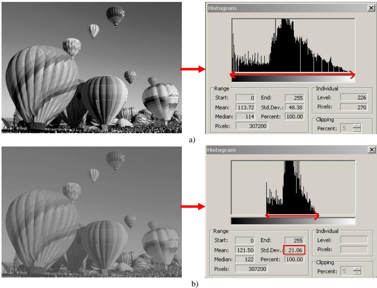
**Fig. 8.13** The position of the histogram and of the standard deviation ( $2\sigma$ ) of the intensity levels for an image of high contrast (a) and an image of low contrast (b)
