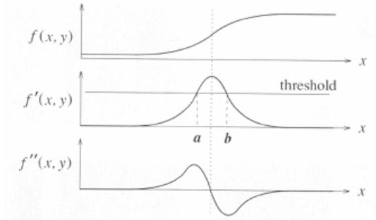
Fig. 11.1 Detection methods of the edge points (points where the image intensity suffers a steep variation)
