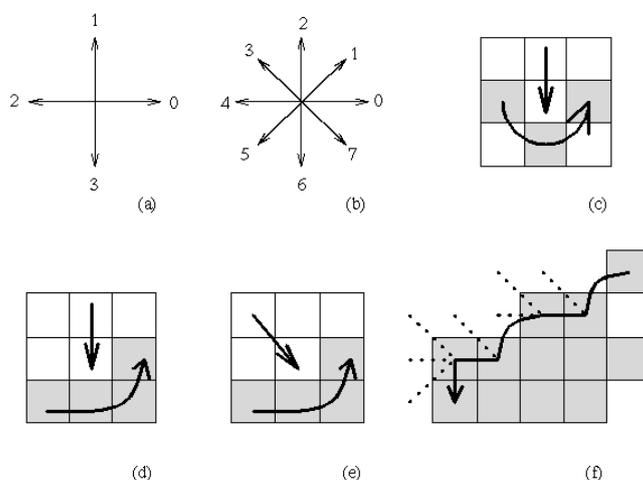
**Fig. 6.1** (a) Direction notation, 4-connectivity, (b) 8-connectivity, (c) pixel neighborhood search sequence is 4-connectivity, (d), (e) search sequence in 8-connectivity, (f) boundary tracing in 8-connectivity (dashed lines show pixels tested during the border tracing) [3]
