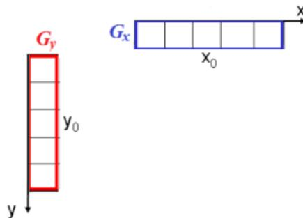
Fig. 10.5 The two vectors  $G_x$  and  $G_y$  into which a 2D Gaussian kernel may be separated
