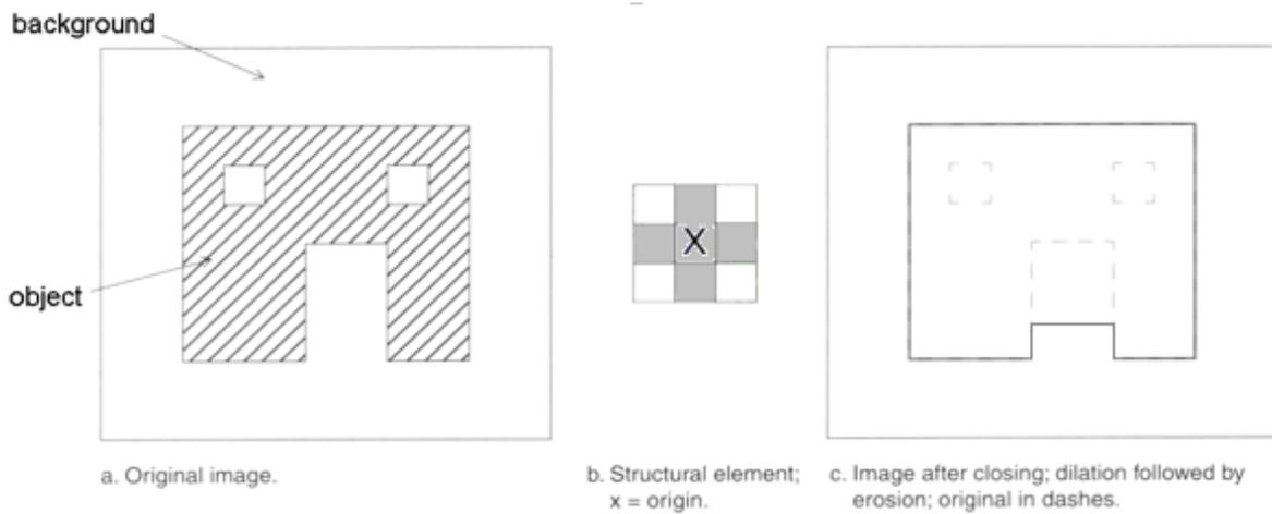
**Fig. 7.7** Illustration of the closing process [1]
