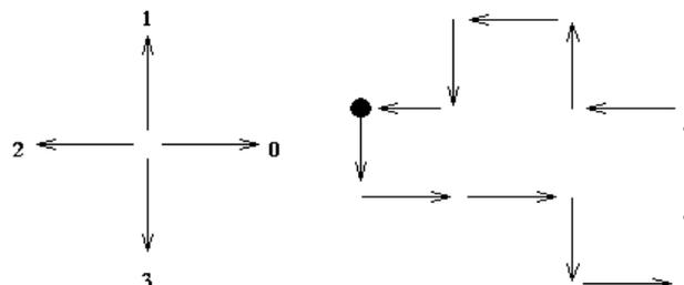
Fig. 6.4 Chain code in 4-connectivity and its derivative
