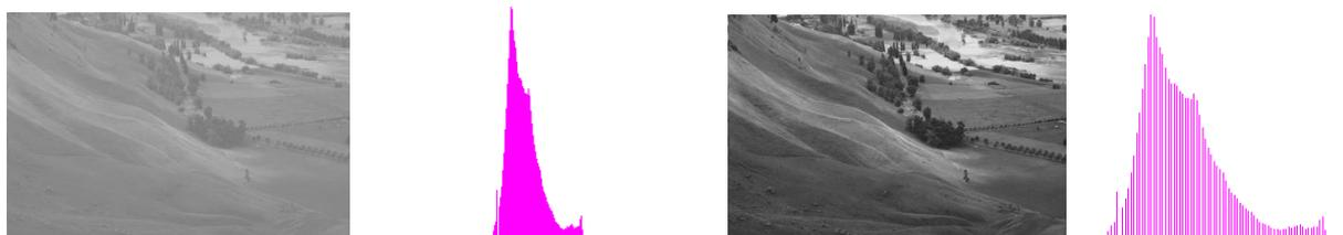
a. Original image and histogram      b. Histogram stretching ( $g_{out}^{MIN}=10, g_{out}^{MAX}=250$ )
