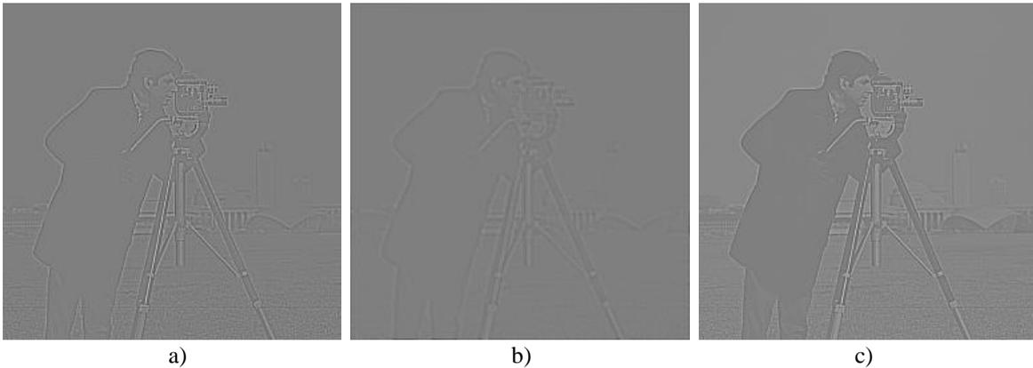
**Fig. 9.3** a) The result of applying the Laplace edge detection filter (9.8) on the original image (Fig. 9.2a); b) The result of applying the Laplace edge detection filter (9.8) on the blurred image from Fig. 9.2b (previously filtered with the 3x3 mean filter); c) The result obtained by filtering the original image with the high-pass filter (9.10)
