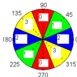
Fig. 11.3 Quantization of the gradient directions in the non-maxima suppression step [3]
