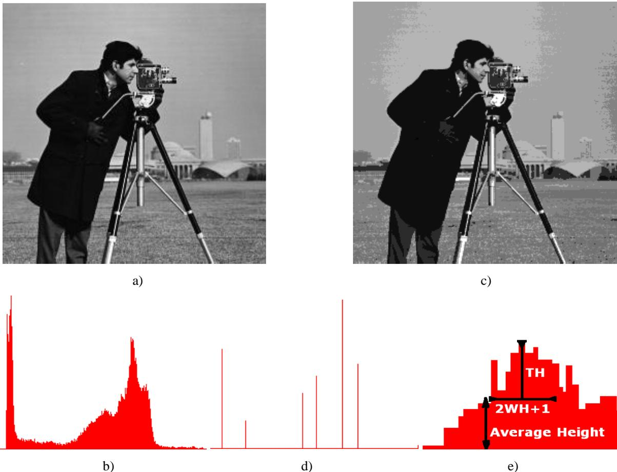
**Fig. 3.2** a) The initial image; b) The histogram of the initial image; c) The obtained multilevel thresholded image; d) The histogram of the multilevel thresholded image; e) The histogram maxima computation algorithm
