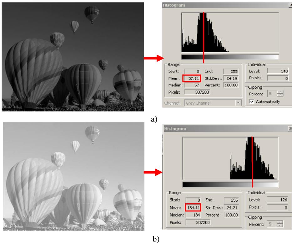
**Fig. 8.12** The position of the histogram and the mean value of the intensity levels for a dark image (a) and a bright image (b)
