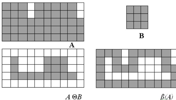
Fig. 7.9 Illustration of the boundary extraction algorithm
