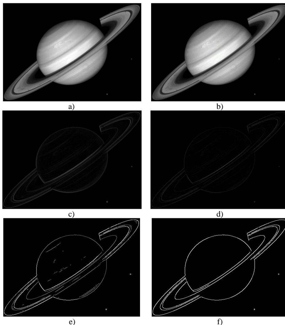
**Fig. 11.6** Canny edge detection - sample results: a) Initial image; b) After Gaussian filtering ( $\sigma = 0.5$ ); c) Normalized gradient magnitude (using Sobel operators); d) After non-maxima suppression; e) After adaptive thresholding ( $p = 0.1$ ); f) Final edges after edge extension with N8 and weak-edge removal
