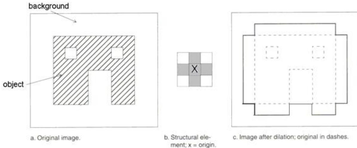
Fig. 7.2 Illustration of the dilation process [1]
