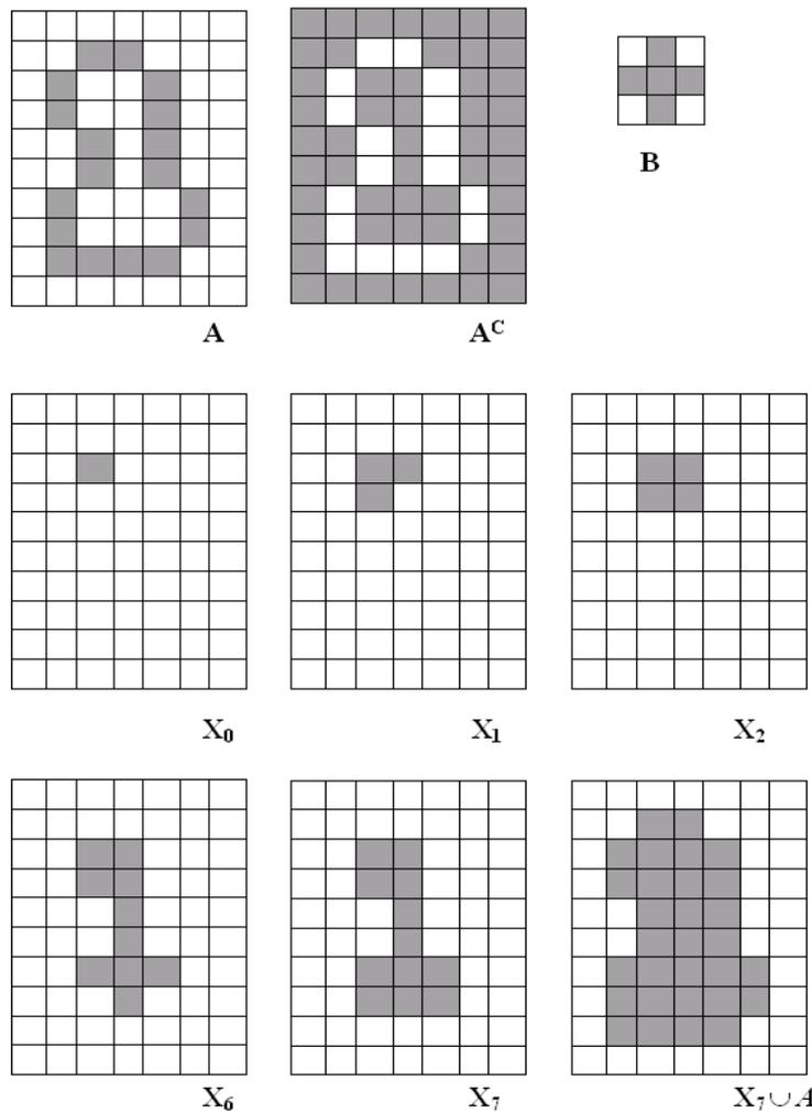
Fig. 7.11 Illustration of the region filling algorithm
