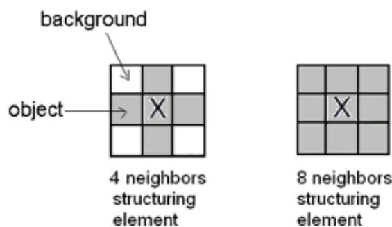
Fig. 7.1 Typical shapes of the structuring elements **B**
