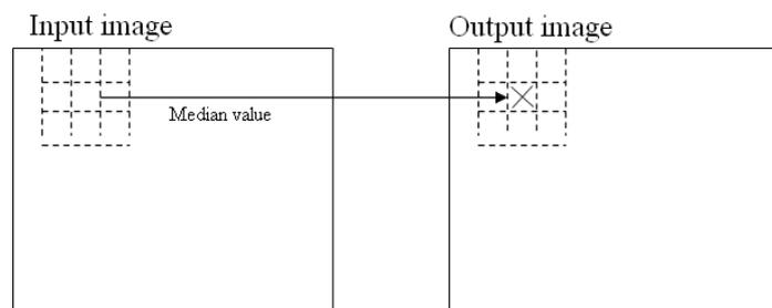
**Fig. 10.3** Applying the median filter
