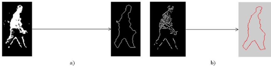
**Fig. 3.** a) Contour extraction (right) on binary image of pedestrian connected components (left). b) Edge image of pedestrian (left) and smoothed contour on edge image using snake (right)
