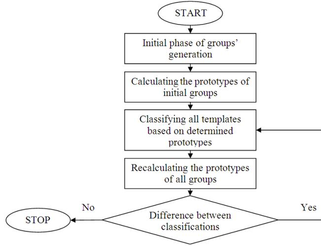
**Fig. 5.** Template tree hierarchy building algorithm at each level of the tree
