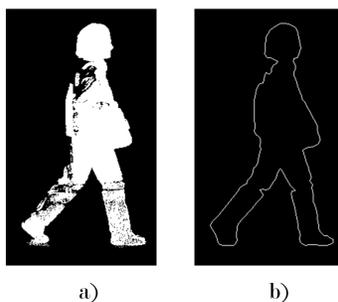
**Fig. 1.** Pedestrian contour extracted from images with fix background: a) Confidence image. b) The extracted contour
