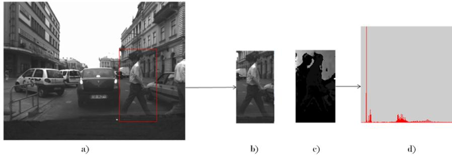
**Fig. 2.** Selection of pedestrian area and depth histogram computation: a) Scene image from a sequence with pedestrian selected area (red). b) Pedestrian selected area. c) Depth image of the pedestrian selected area (red). d) The computed depth histogram.
