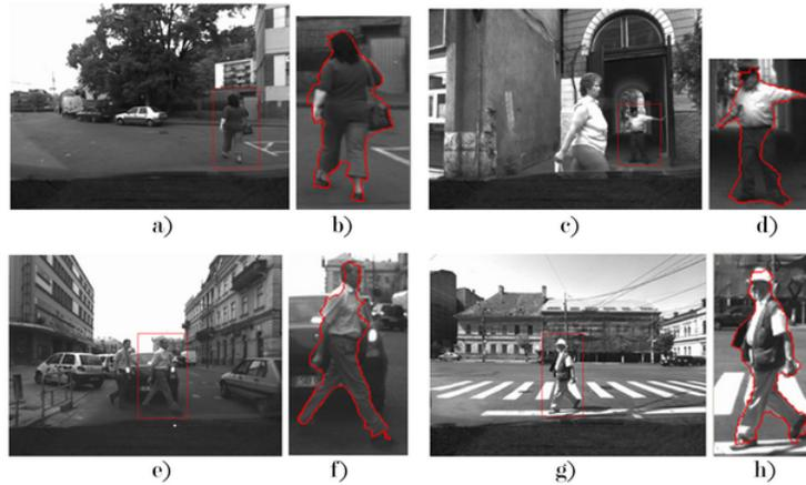
**Fig. 8.** Pedestrian contour extracted from scene image with dynamic background: a), c), e), g) Scene image and pedestrian selected area. b), d), f), h) The extracted contour of the corresponding pedestrian.
