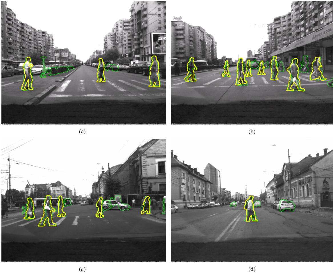
Figure 9. Objects classified as pedestrians (full body contour based matching)
