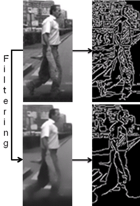
Figure 5. An original and filtered object (left) and corresponding extracted edges (right)
