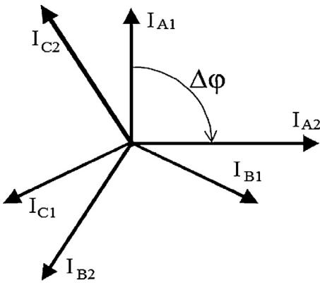
**Fig. 5.** Phase shift between EPL circuits.
