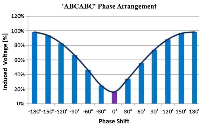
Fig. 7. Induced voltage with respect to no phase shift case for different phase shifts for the 'ABCABC' phase arrangement.
