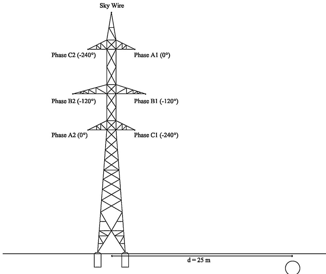
Fig. 3. Cross section of the common distribution corridor.
