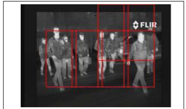
Fig. 4. Snapshot of the program detecting all the pedestrians from an IR image
