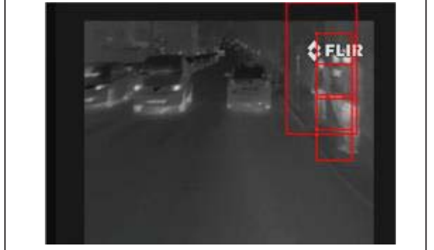
Fig. 5. Snapshot of the program detecting pedestrians using ADA Boost with decision stump classifier
