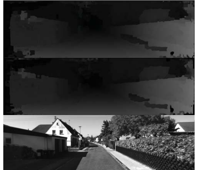
Fig. 5. Bottom image is the left intensity image, in the second image the output of our algorithm is presented, in the first image the result of the census algorithm without our optimization is illustrated.
