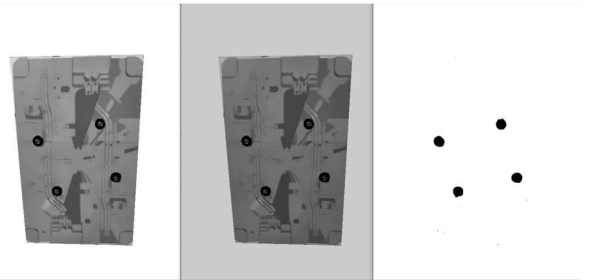
Figure 5. In the left image, the original ROI is shown, the middle image corresponds to the ROI after the contrast and brightness adjustments, the right image illustrates the identified bushing location
