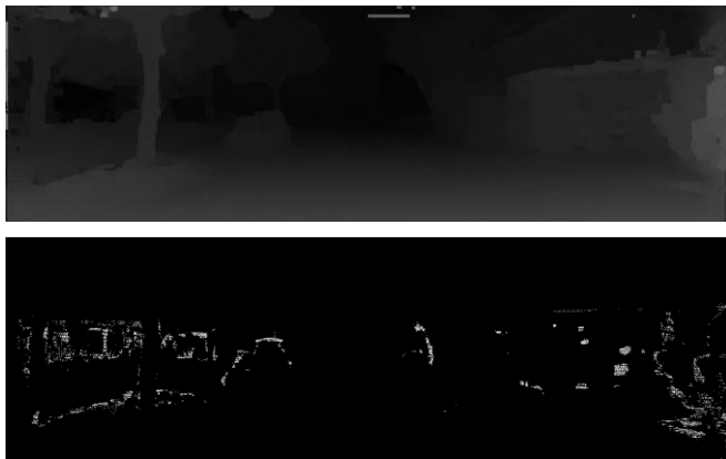
Figure 3. Disparity map of the proposed fusion and its error map using a 2-pixel threshold of a KITTI image
