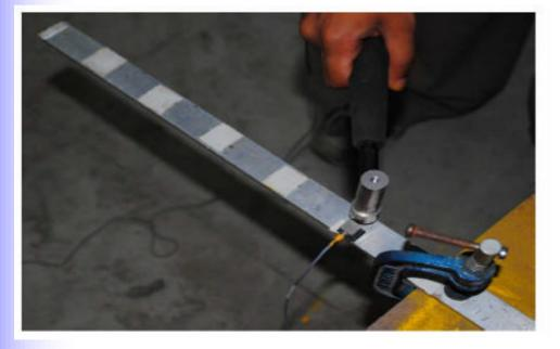
a) Impulse hammer; b) eccentric mass vibrator;c) electrodynamic shaker over three load cells;d) impulse excitation device for bridges
