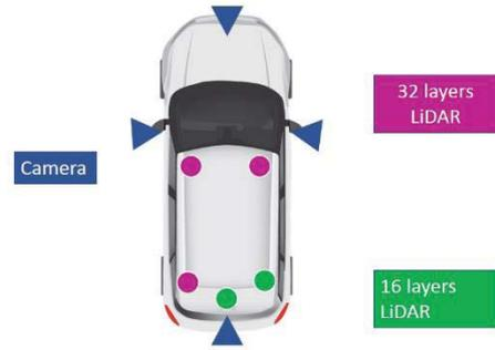
**Fig 5. Vehicle's sensors infrastructure.**
