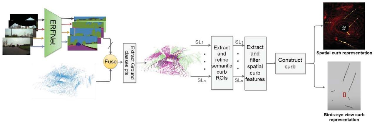
**Fig. 1. The processing pipeline of the proposed system.**
