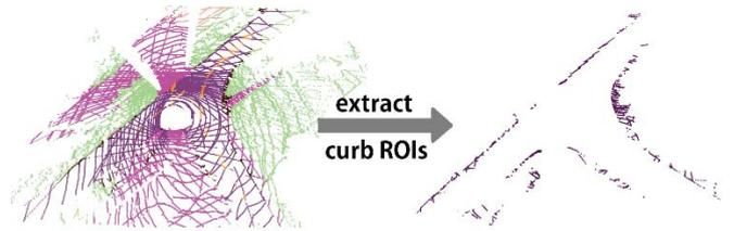
Fig. 2. Obtaining the unrefined curb ROIs.
