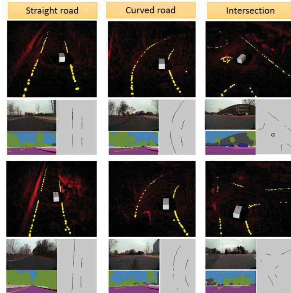
**Fig. 6. Results of the proposed method for different types of urban road scenarios.**
