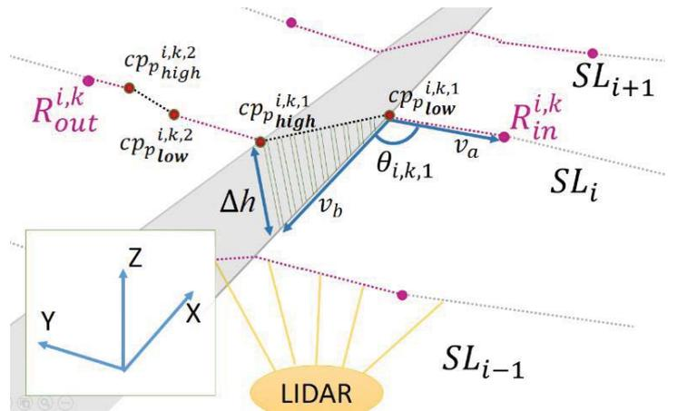
**Fig 4. Candidate curb transversal regions illustration extracted using spatial features.**
