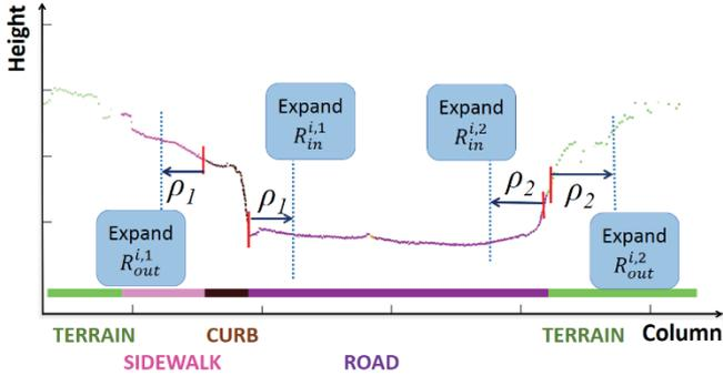
**Fig. 3. Expanding curb ROIs for a LiDAR scan line.**
