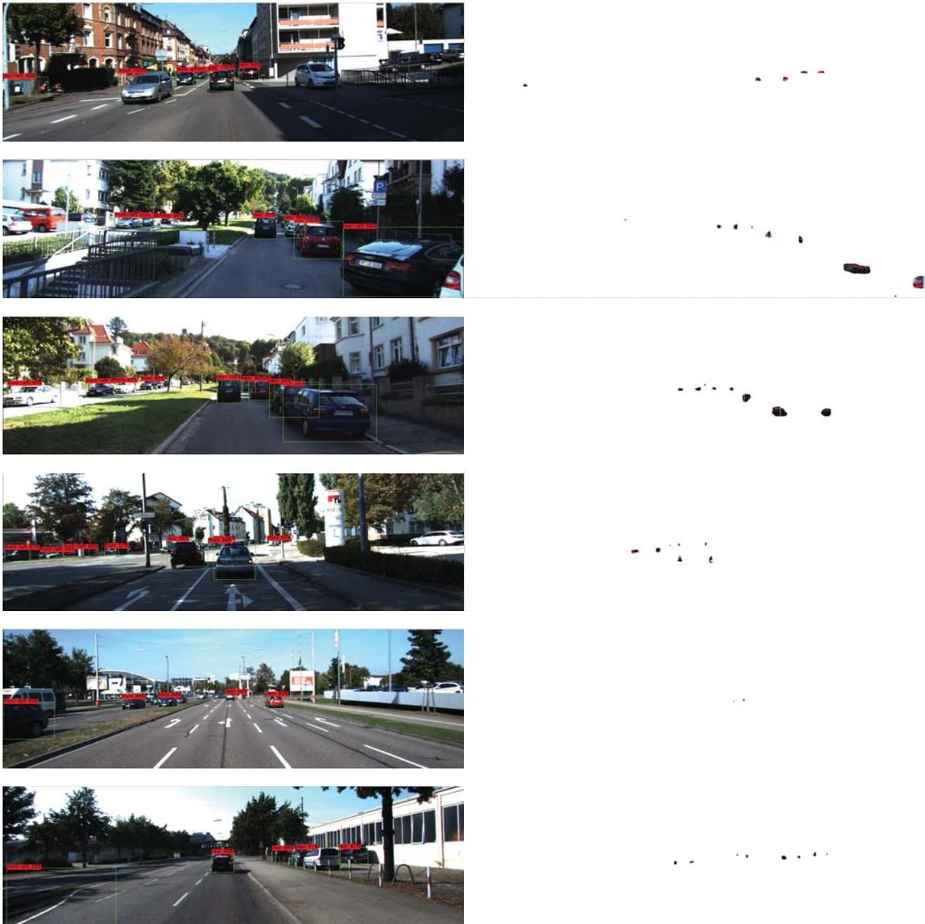
Fig. 4. Network results with ERFNet as a base network. Left column: vehicle and orientation detection. Right column: taillight segmentation.
