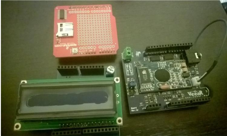
Since the Arduino boards are very popular, many competitors are using the same design layout (see the figure bellow: left - a Fez Domino board with ARM processor; right- a CipKit board with PIC processor) being also able to use the Arduino compatible shields.
