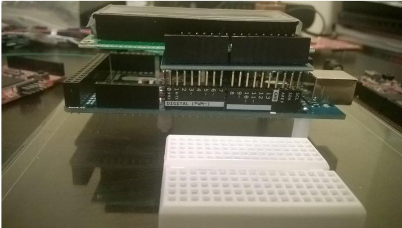
**The LCD uses the digital pins 2 ... 7:** 7 – RS, 6 – En, 5 – DB4, 4 – Db5, 3 – DB6, 2 – DB7 (their mining is in the table bellow).
