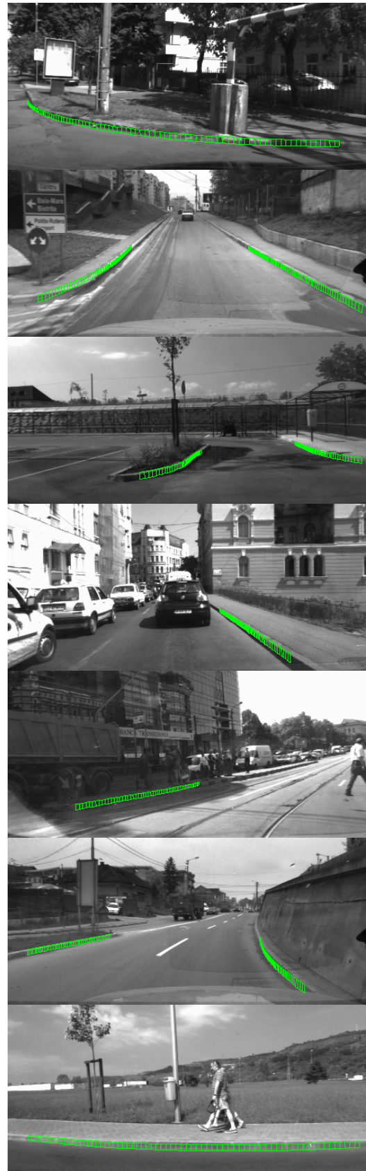
Fig. 11. Results of the proposed polynomial curb detection algorithm. Various road geometries are present, including a 10% uphill (second image from the top).
