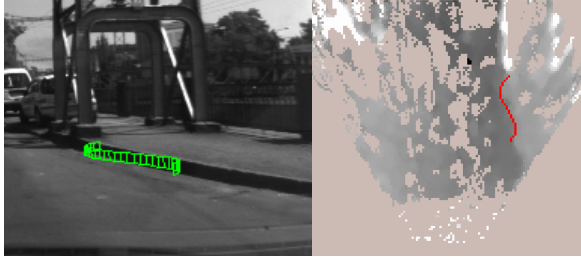
Fig. 10. Example of unstable polynomial curve caused by bad 3D data. Even though the real 3D curb is straight, the DEM curb “looks” undulated.
