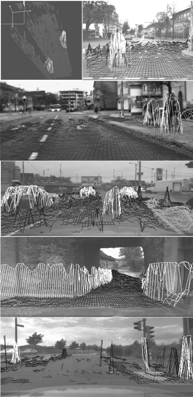
Fig. 11. Results for various scenes. The algorithm performs well even for scenes with sparse 3D road reconstruction and noisy 3d data (the grid is projected only where dense 3D data is provided by the dense stereo engine). The result for the first scene is displayed using a virtual camera. Grid colors represent dark gray - road, gray - traffic isle, and white - obstacles.
