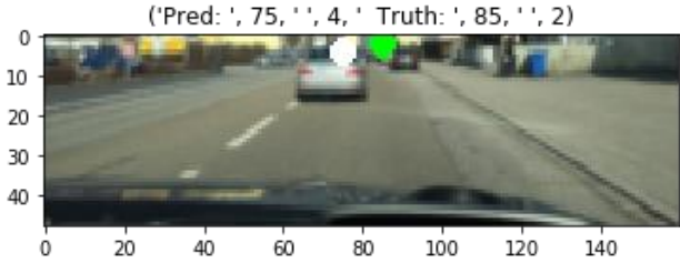
Fig. 8. Example of a predicted vanishing point that is better than the vanishing point computed by traditional algorithms. The green circle represents the ground truth and the white circle is the prediction.
