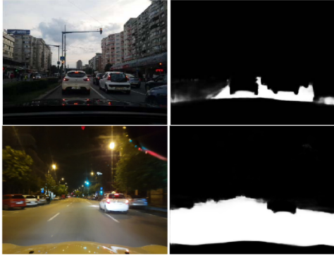
Fig. 9. Example of predictions in complex city scenarios during day time and night time.
