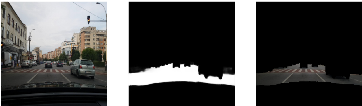
Figure 1. Example of semantic segmentation using the artificial network.
