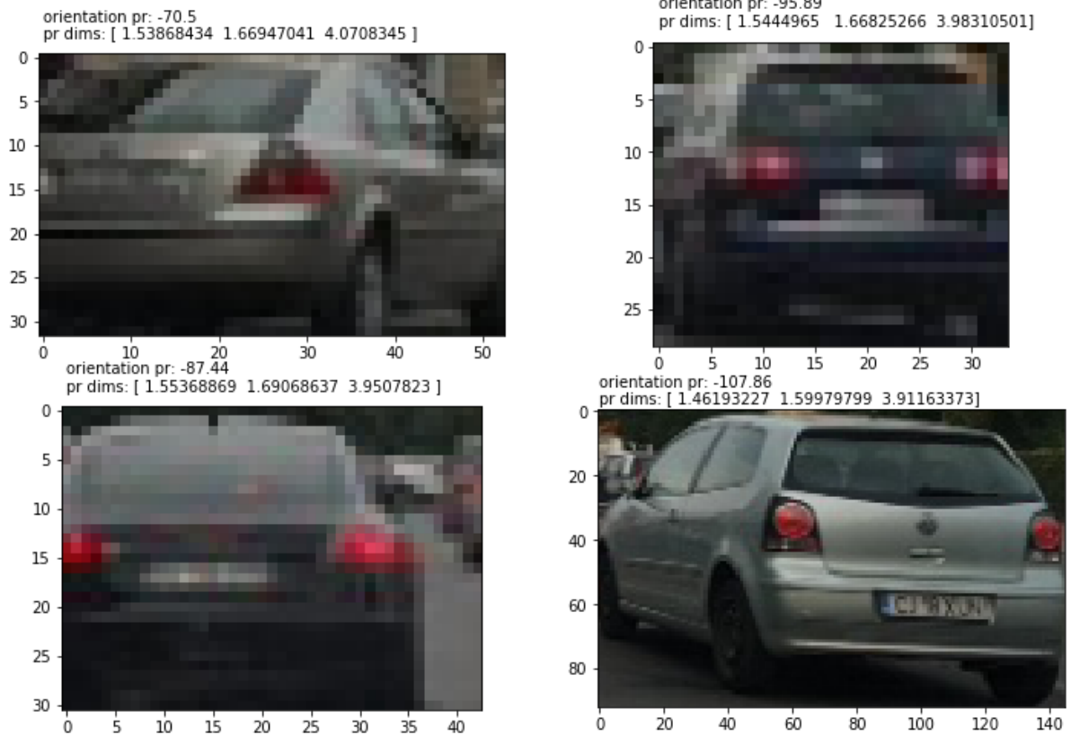
Figure 6. The predictions for vehicle orientation and dimensions.
