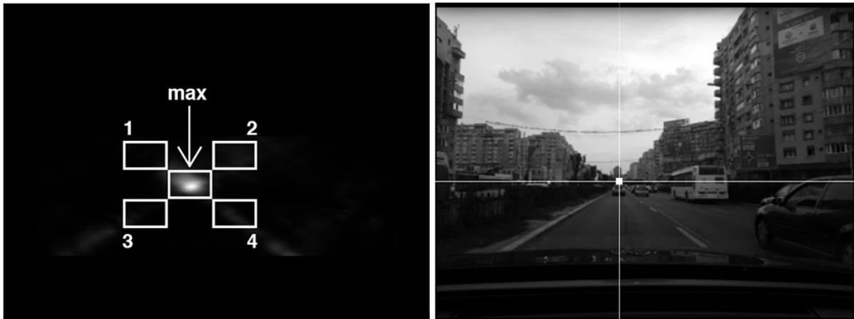
Figure 8. Left: the window with the most votes (max) from the vote map along with the validation windows that are used (numbered 1 to 4). Right: The final result of the algorithm with the computed vanishing point.
