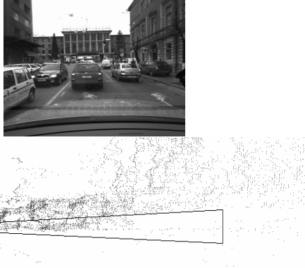
Fig. 2. A complex city scene with road, cars and walls, and a side view of the reconstructed 3D points. The possible domain of pitch variation is highlighted.
