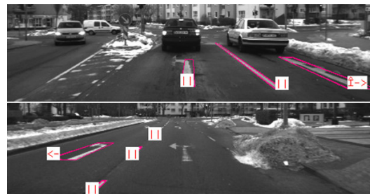
Fig. 20. Results – errors in classification. Top – left arrow misclassified as lane marking, due to partial visibility; Bottom – arrow completely missed due to low visibility.
