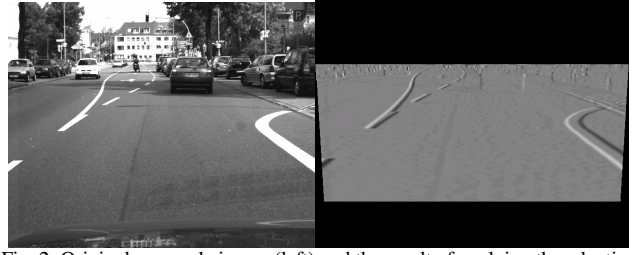
Fig. 2. Original grayscale image (left) and the result of applying the adaptive horizontal gradient filter (right)
