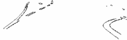
Fig. 4. Extracted lane marking edges
