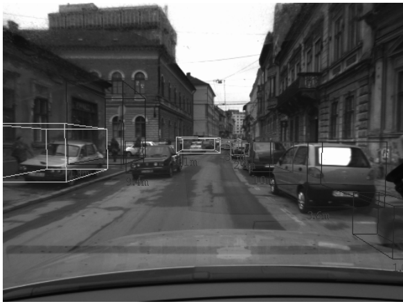
Fig. 1. Grouping the 3D points into cuboids – perspective view
