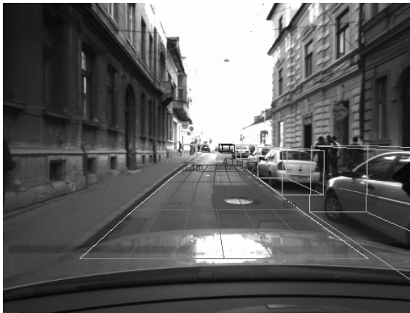
Fig. 11. Tracking results – the side objects are correctly tracked as we pass them.
