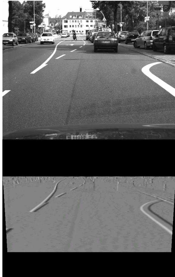
Fig. 3. Original grayscale image (top) and the result of applying the adaptive horizontal gradient filter (bottom)
