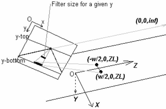
Figure 2. Computing the width of the differentiation filter
