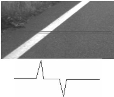
**Figure 1. The horizontal gradient for a lane marking. Dark-light-dark transition is encoded in the gradient**
