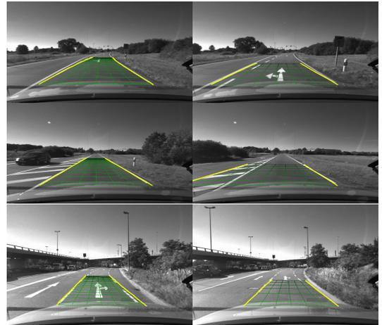
Fig. 11. Samples of side by side comparison. Left – particle filter solution, Right – Kalman filter solution.
