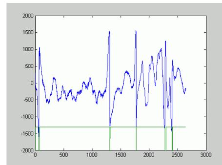
Fig. 15. Highway behavior: lateral offset (distance of the vehicle from lane center, in mm) versus frame number.
