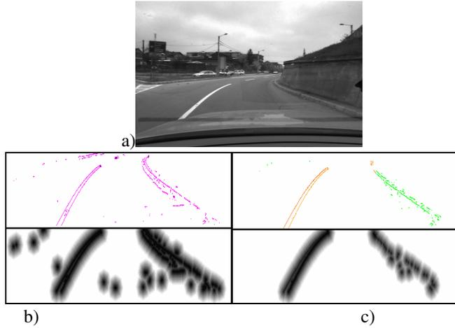
Fig. 9. Visual information: a) the original grayscale image, b) the edges corresponding to 3d points contained in the road surface and the associated distance transform image, c) markings and curbs, and their associated DT image
