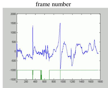
Fig. 19. Urban behavior: lateral offset (distance of the vehicle from lane center, in mm) versus frame number
