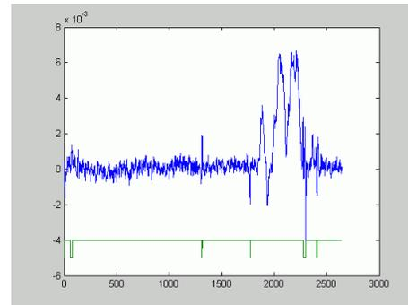
Fig. 14. Highway behavior: horizontal curvature ( $m^{-1}$ ) versus frame number.
