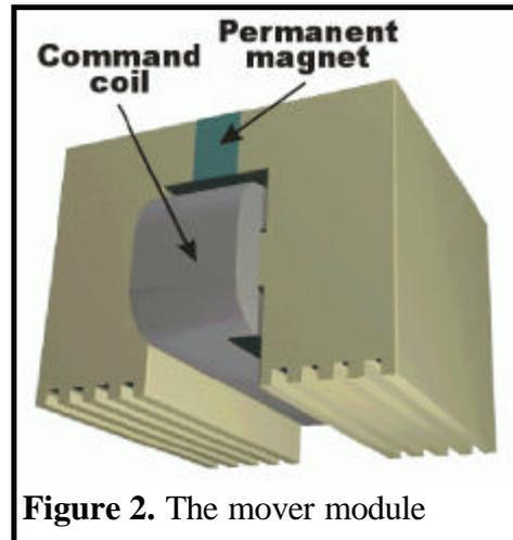
**Figure 2.** The mover module
