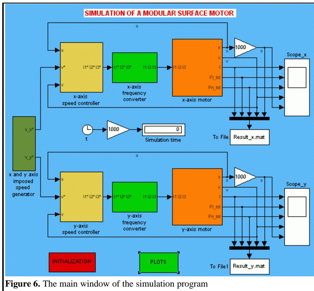
Figure 6. The main window of the simulation program
