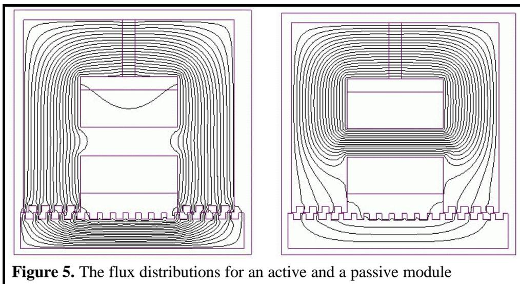
**Figure 5.** The flux distributions for an active and a passive module
