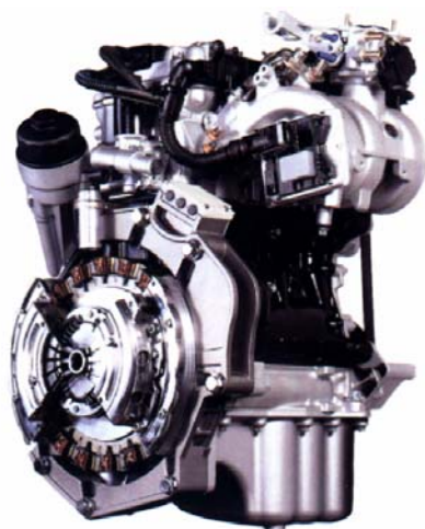
Fig. 14. Car engine equipped with a crankshaft starter-alternator
