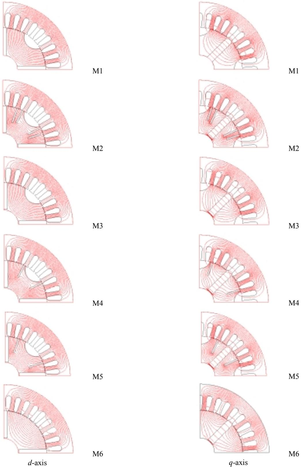
Fig. 2. The  $d$ - and  $q$ -axis flux plots for M1-M6 rotor variants
