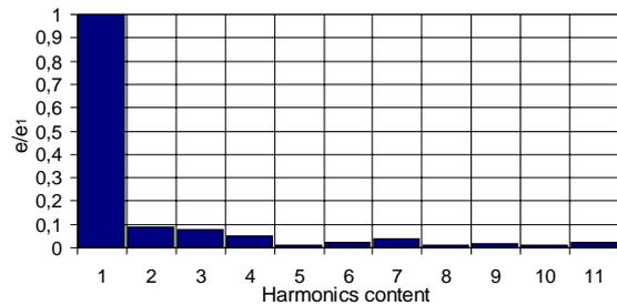
Fig. 8. Phase  $c$  EMF harmonics content on the rotor  $d$ -axis
