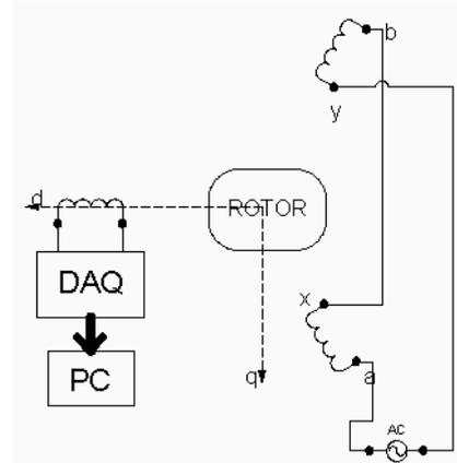
Fig. 7. Test set-up to evaluate the harmonics
