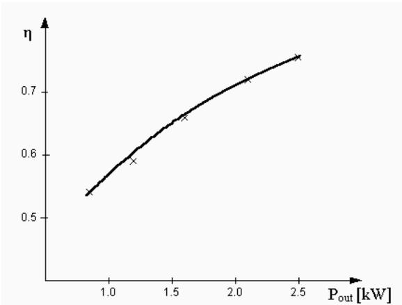
Fig. 6. Efficiency versus output power
