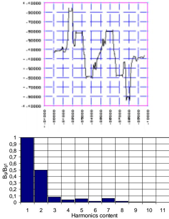
Fig. 4. The air-gap flux density variation on a pole pitch and the corresponding harmonic spectrum for  $q$ -axis
