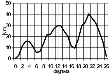
Fig. 5. The electromagnetic torque variation function of the rotor position
