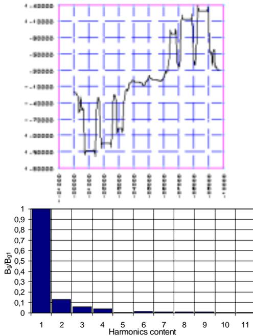
Fig. 3. The air-gap flux density variation on a pole pitch and the corresponding harmonic spectrum for  $d$ -axis
